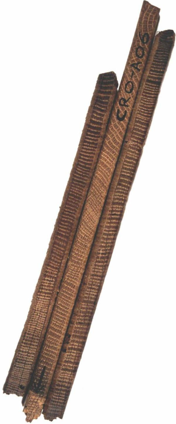
*Figure A4: Three cores from timbers in a building. They come from trees growing at the same time. Notice that, although the sequences of widths look similar, they are not identical. This is typical*
