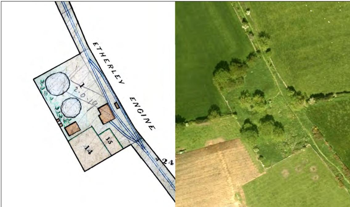
Fig 11: The Etherley Engine consisted of the Engine House, the Engineman's House and two ponds to supply the water for the steam engine. All that is visible on modern aerial photographs are the partly levelled earthworks of the southern pond and the enclosure wall. Left: 1839 Thomas Dixon plan. Source: Archaeo-Environment Ltd. Reproduced with kind permission of The National Archives, ref. RAIL 1037/451; Right: NZ1728 11-JUN-2015 © Bluesky International/Getmapping PLC.
