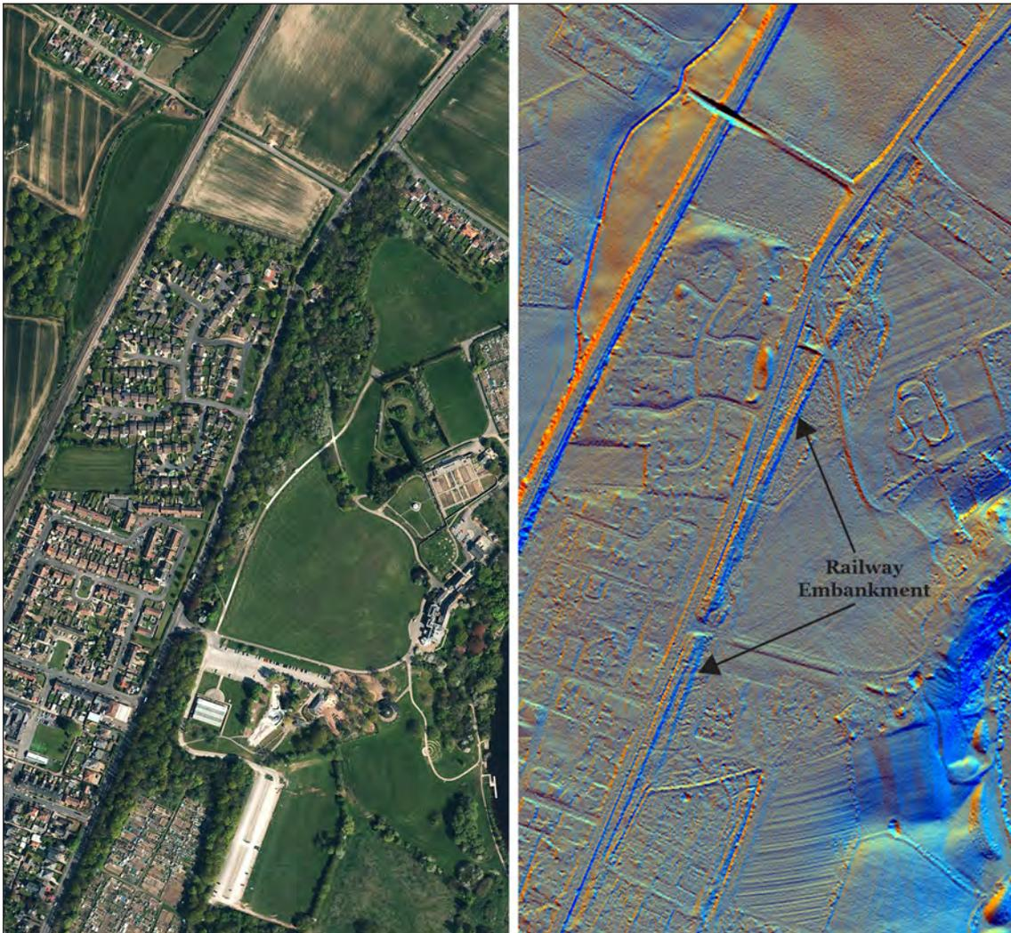
*Fig 35: The Yarm to Bowesfield stretch of the railway was abandoned in 1853, but the earthwork remains of the embankment can still be traced in woodland in Preston Park. Left image: NZ4215-4316 09-MAY-2016 © Bluesky International/Getmapping PLC; Right image: LIDAR DTM FEB-2011 © Historic England; source Environment Agency.*
