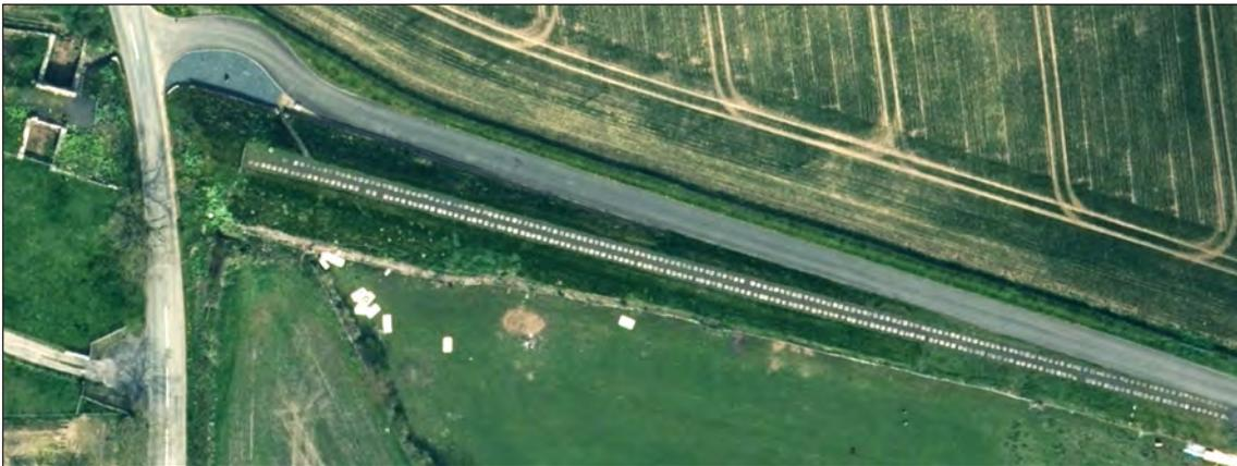
*Fig 81: Where the S&DR spanned Brusselton Lane is the only place in the project where the original stone sleepers were visible on aerial photographs. They were exposed recently by a local volunteer group and are not visible on historic aerial photography. Detail of NZ2125 06-MAY-2016 © Bluesky International/Getmapping PLC.*
