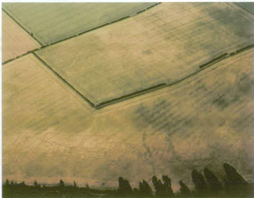
Figure 2 Crop marks on the plateau immediately above South Common marking the presence of fissures in the underlying limestone (NMR 12855/08 ©Crown copyright. NMR).
