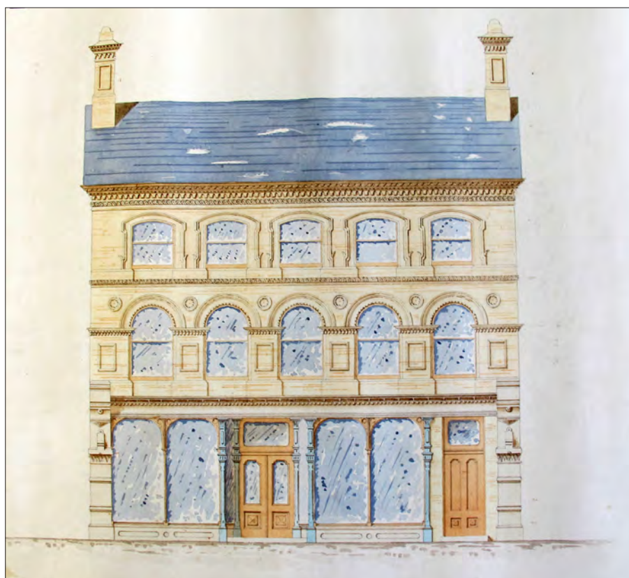
Figure 99. Proposed elevation of 99 High Street as designed by W. O. Chambers in 1866. The surviving fabric of 99 High Street suggests that the building was largely built as designed here. Reproduced by kind permission of Suffolk Record Office, ref SROI: HG3/1/2/56 (detail)
