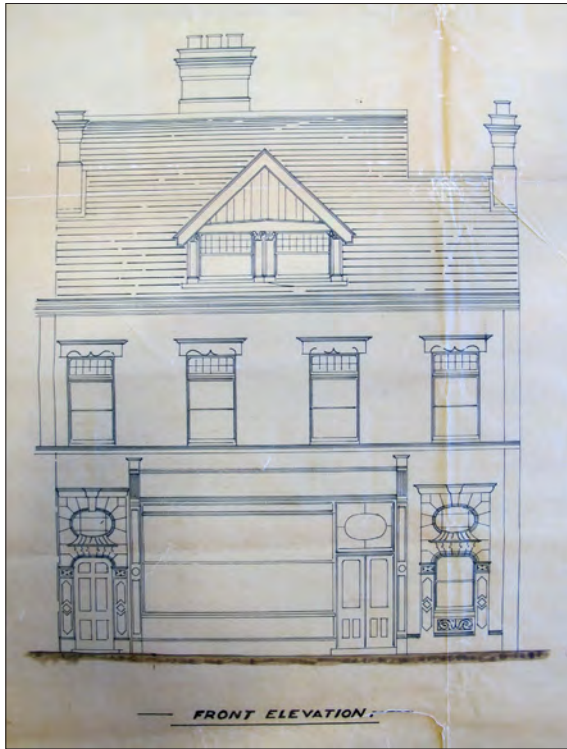
Figure 138 (left). 133 High Street was designed by W. J. Roberts in 1903 with an inscribed marble stallriser, a contemporary take on the traditional design for a butchers' shop. SROL: 98/2753. Reproduced courtesy of East Suffolk Council
