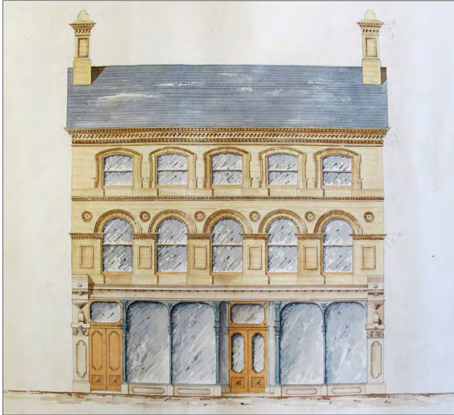
Figure 100. Alternative design by W. O. Chambers for 99 High Street, showing a largely cast-iron shopfront. Reproduced by kind permission of Suffolk Record Office, ref SRO: HG3/1/2/56 (detail)
