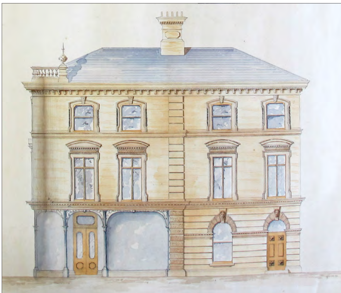
Figure 127. 1864 designs by W. O. Chambers for a grocer's shop on the corner of the High Street and St Peter's Street show an Italianate building with a cast-iron shopfront. Reproduced by kind permission of Suffolk Record Office, ref SROI: HG3/1/2/69 (detail)
