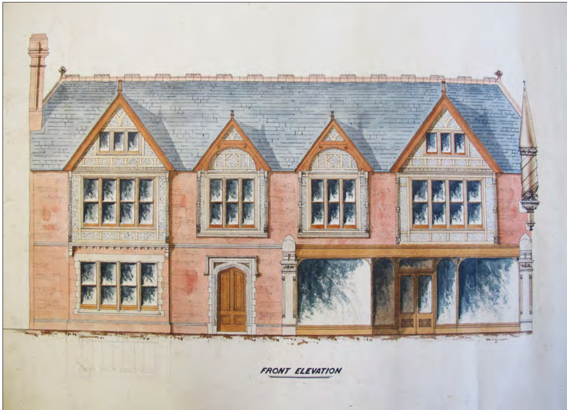
Figure 90. Elevation drawing of proposed alterations at 90-91 High Street by W. O. Chambers, c.1880. Reproduced by kind permission of Suffolk Record Office, ref SROI: HG3/1/2/190
