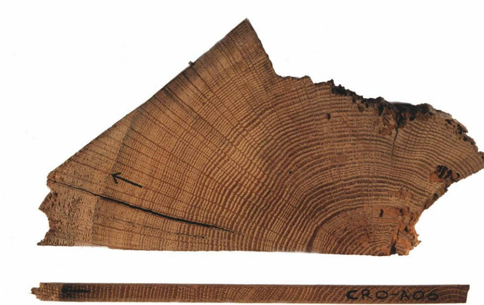
Figure A2: Cross-section of a rafter, showing sapwood rings in the left-hand corner, the arrow points to the heartwood/sapwood boundary (H/S); and a core with sapwood; again the arrow is pointing to the H/S. The core is about the size of a pencil
