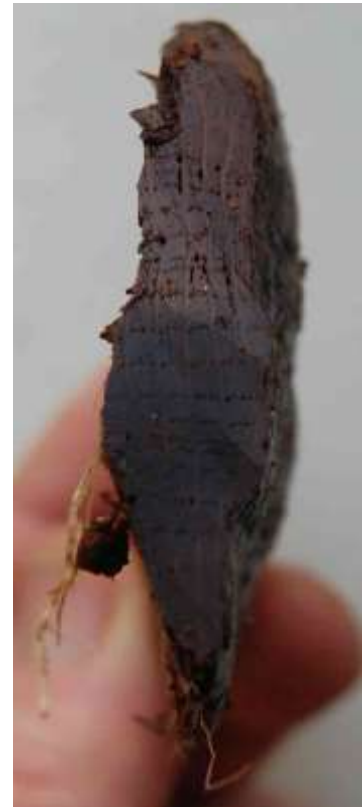
Figure 85 shrinkage of sapwood -lighter colour at top
