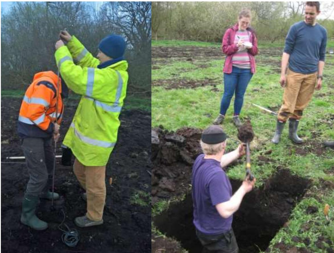
Figure 30. Oxygen and temperature sensors were installed from the soil surface through a removable installation tube (left). A small test pit was dug outside the membrane covered area to take ring samples of soil for porosity measurements (right)
