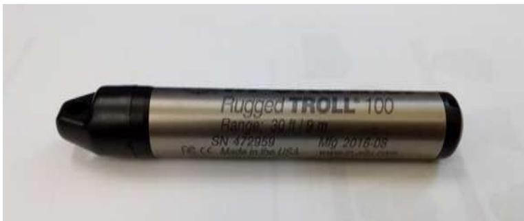
Figure 33: The Rugged TROLL™ 100 transducer.
