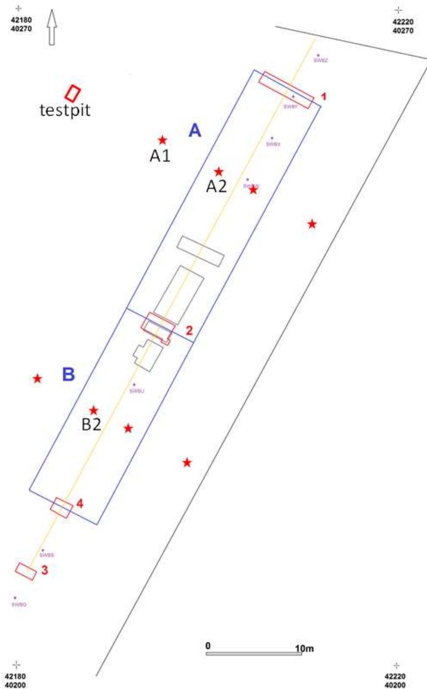
Figure 31. Map of site with location of monitoring equipment and test pit. Blue line: location of plastic membrane. Red stars: approximate location of dipwells. Oxygen, temperature and water content sensors were installed within 1 m of dipwells A1, A2 and B2.
