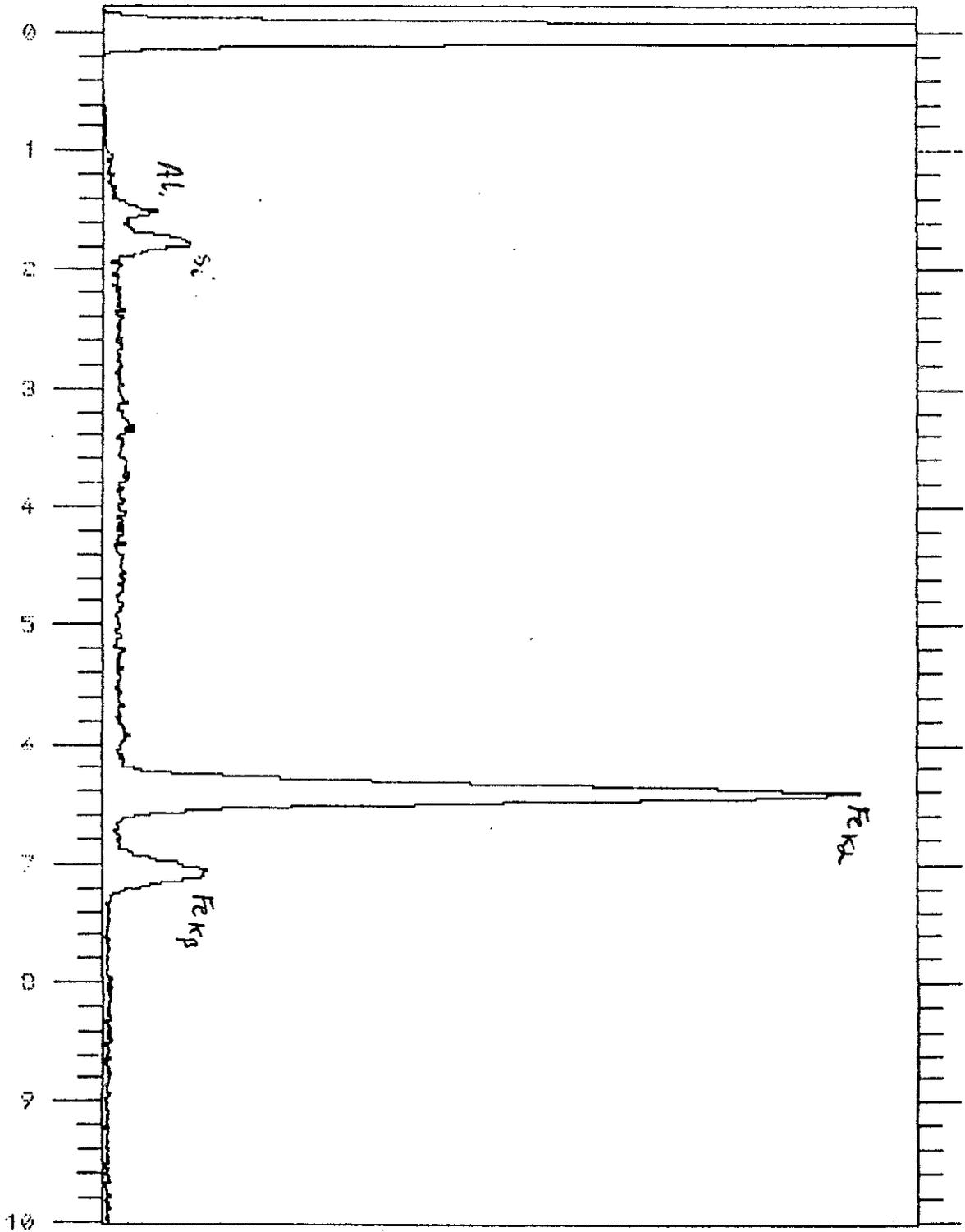
FIGURE 3 Qualitative EDS X-ray Analysis of hematite
