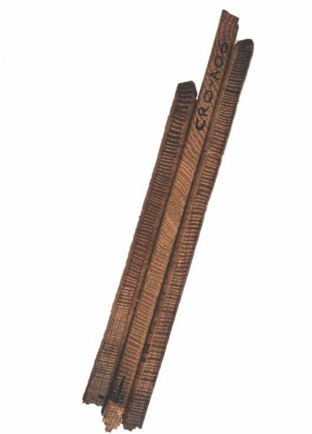
Figure A4: Three cores from timbers in a building. They come from trees growing at the same time. Notice that, although the sequences of widths look similar, they are not identical. This is typical
