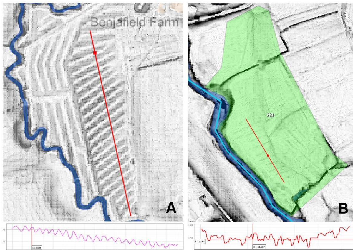
Figure 10A Profile across area of bedworks water meadow on the River Shreen, north east of Gillingham. Contrasts with Figure 10B, HWP 221 near Sturminster Newton which shows an area of faintly identifiable bedworks water meadow present on the SVF processed lidar.
