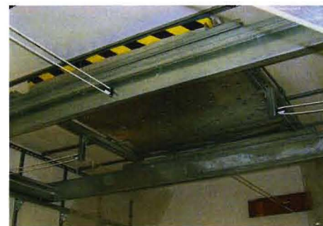
Photo: Underside of water tank with perforated base of the new BRE rain noise measurement rig. (Source: BRE)
