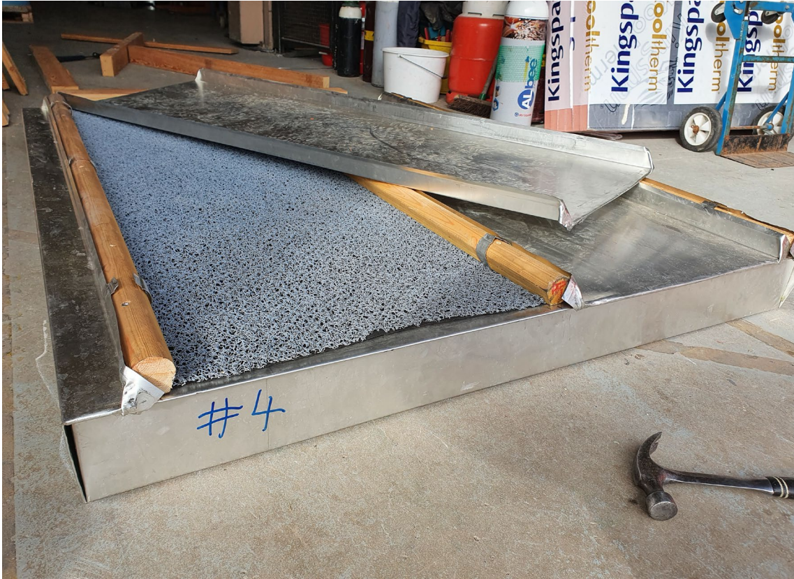
Photo A5: Sample 4 – TCSS batten roll, spiral mesh underlay
