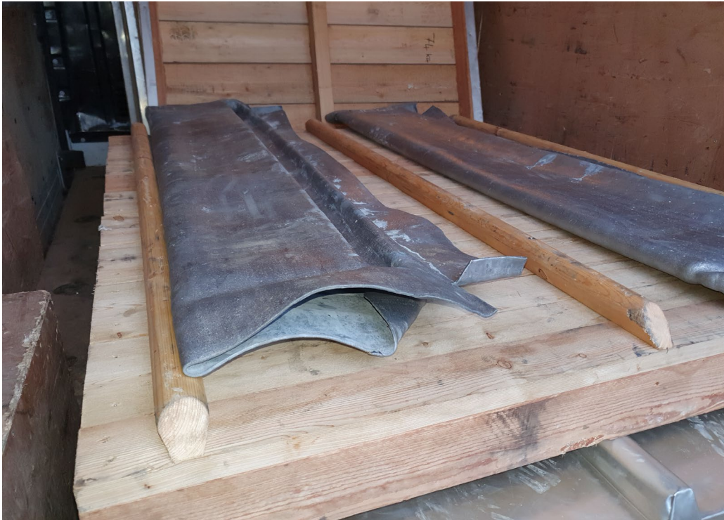
Photo A1: Sample 1 – lead batten roll, no underlay
