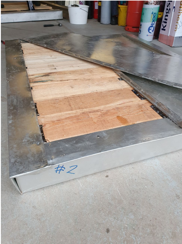
Photo A3: Sample 2 – TCSS standing seam, no underlay
