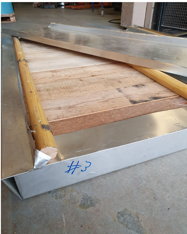
Photo A4: Sample 3 – TCSS batten roll, no underlay
