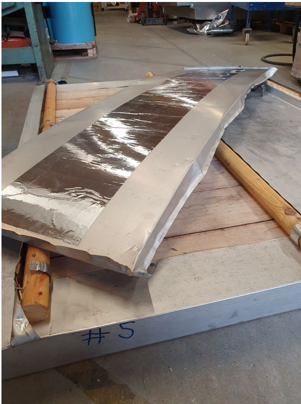
Photo A6: Sample 5 – TCSS batten roll, adhered acoustic mat
