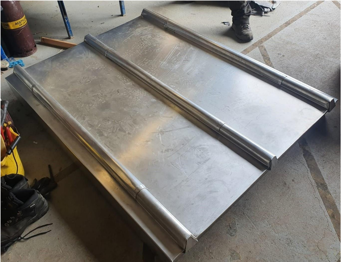
View of 0.5mm TCSS Batten Roll Seam sample
