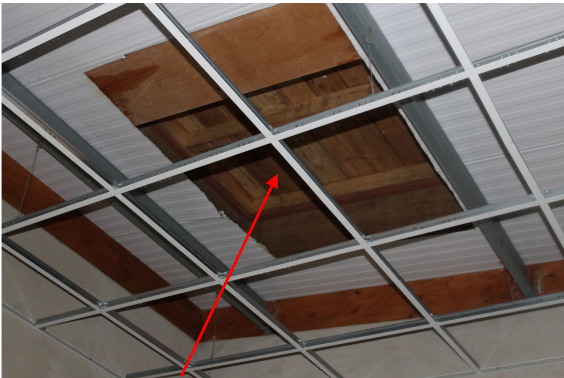
Photo B1: TCSS roof sample mounted on roof of acoustic test room
