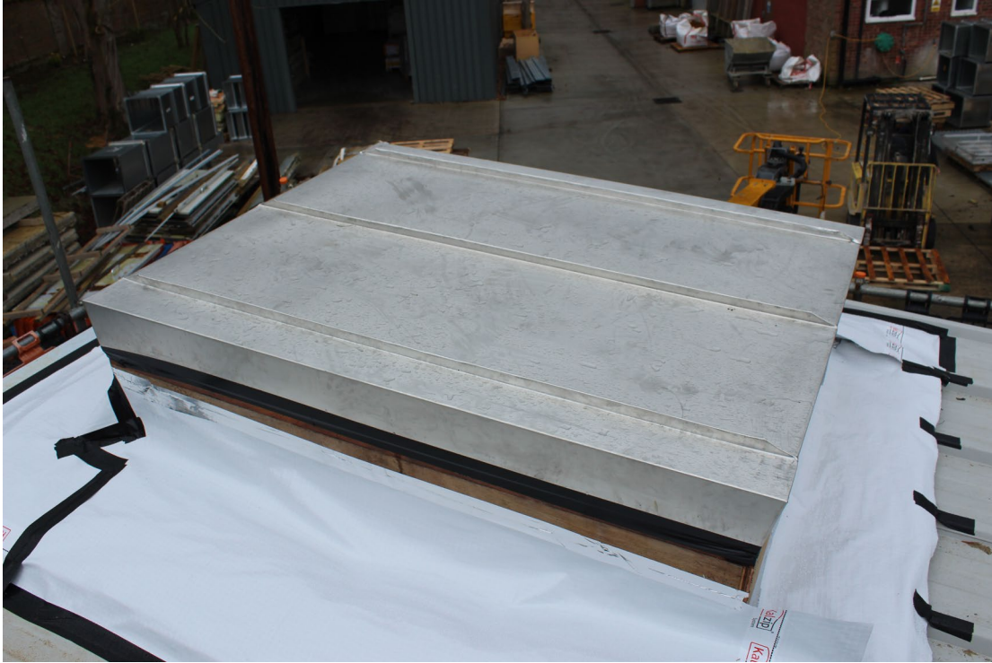
Photo B1: TCSS roof sample mounted on roof of acoustic test room
