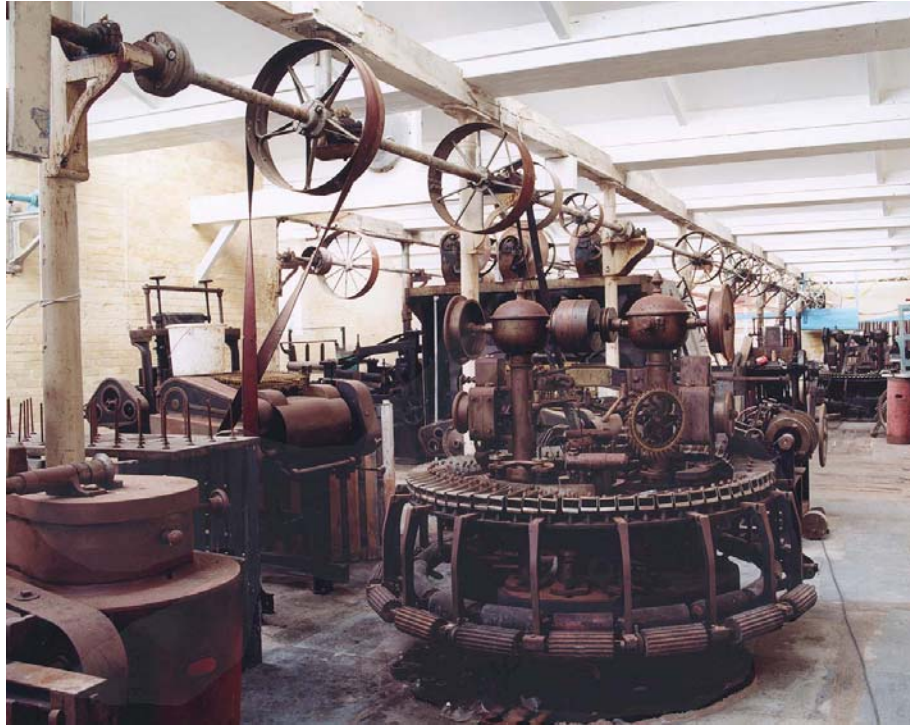
Fig 18. Gill box (left) and Noble comb powered by line shafting in the combing shed.
