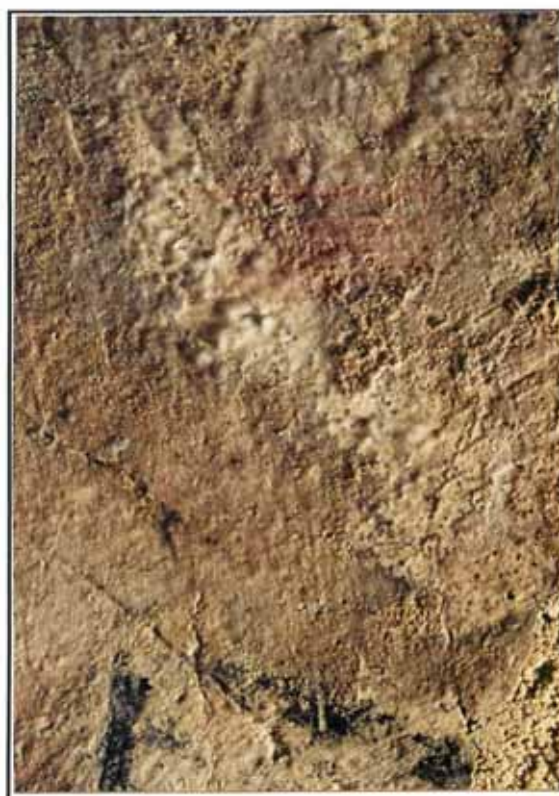
Plate 11: Horsham St Faith Priory; detail of figure of St Faith. The fungus, identified as Cladosporium , generally appears as an off white, patchy, fibrous growth. During the reproductive stage however the fungus turns black. In addition to the serious disruption this causes to the pictorial image, the painted surfaces themselves are attacked by the growth of a vegetative mycelium within the substrate [ see JAMES 1988 ].
