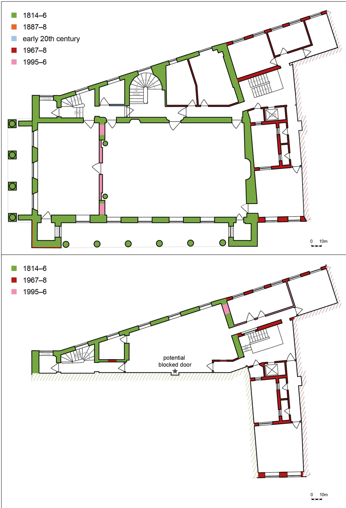
Figures 33 and 34: Plans of the first (above) and second floors, showing the different phases of the building. [Plans based on the asset management floor plans of the Isle of Wight Council's Corporate and Facilities Management team]
