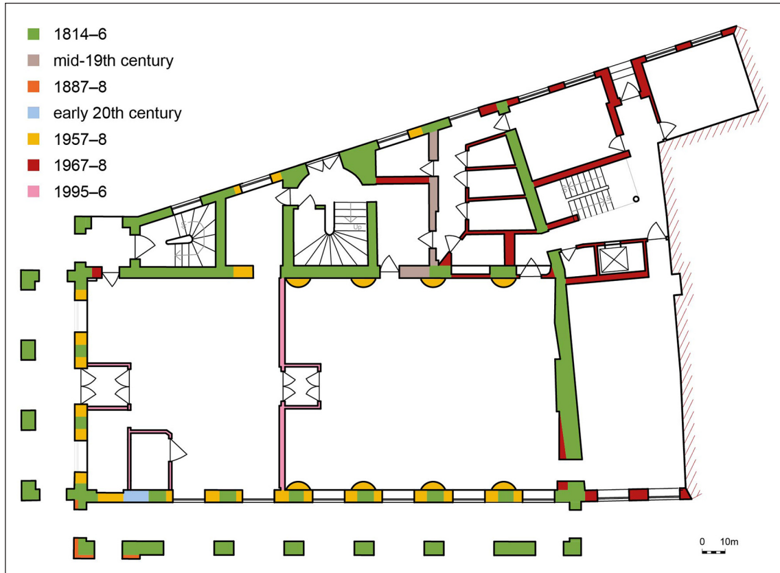
Figure 32: Ground-floor plan showing the different phases of the building. [Plan based on the asset management floor plan of the Isle of Wight Council's Corporate and Facilities Management team]
