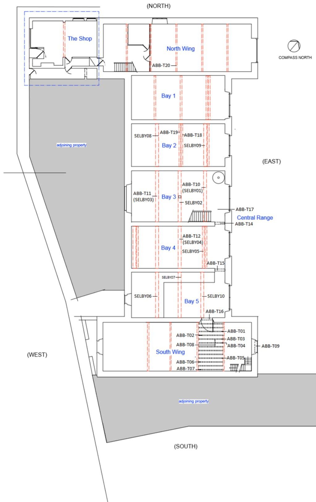
Figure 7: Ground-floor plan, showing sampled timbers, with exception of ex situ beam ABB-T13/SELBY11 (after Wiles & Maguire)
