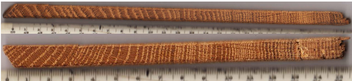
Figure 6: Samples YOR-A05 (top) and YOR-A08 (bottom) showing the cracks and degradation, most apparent in the latter (sapwood) sections of these cores
