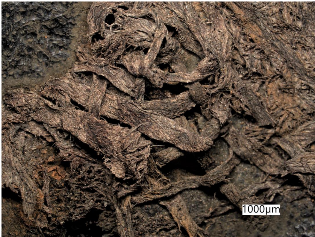
Figure 11: Coarse textile showing the weakly z-twist partly processed plant fibre thread used in its construction. (x120 magnification)
