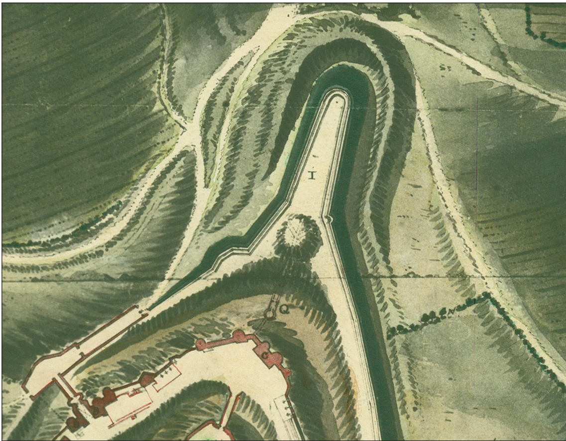
Figure 8 Detail from 1756 Board of Ordnance map. In the inset key, C is described as 'The Main Guard-house'; I as 'An advanced Work finished in July 1756'; and Q as 'A Guard room, for a Sergeants Guard, now erecting on the Sally port into the advanced Work'. Three tunnels are marked in dotted lines within the circular mound on the terreplein. [HE Archive: MP/DOV0030]
