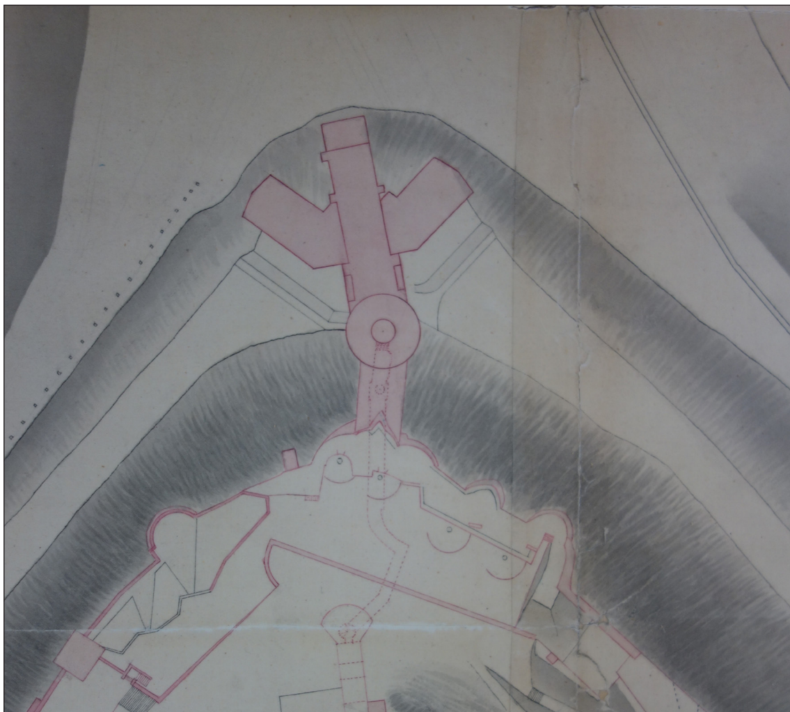
Figure 15 Detail from an undated, possibly 1806 Board of Ordnance plan copied by Thomas Peckham and E.B. Metcalf. It shows the alterations carried out under Twiss, including caponier, casemated wing caponiers (with drop ditches), Spur Casemates and emplacements and the new entrance from Outer Bailey. The redan is indicated in faint pencil. [TNA: MR 1/845. Reproduced with permission].
