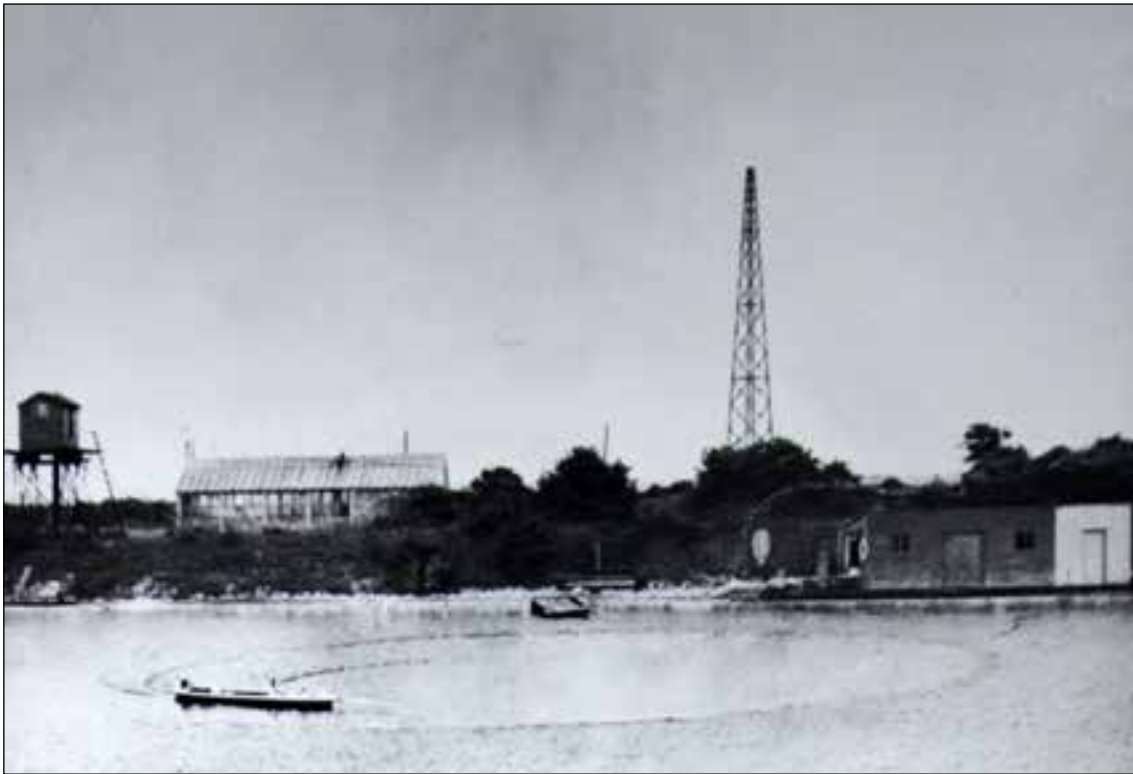
Figure 16: A model ship undergoing manoeuvring tests on Horsea Lake (TNA ADM 1/23580)
