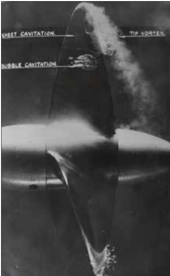
Figure 7: High-speed photograph of a model propeller demonstrating the effects of cavitation (TNA ADM 226/68)
