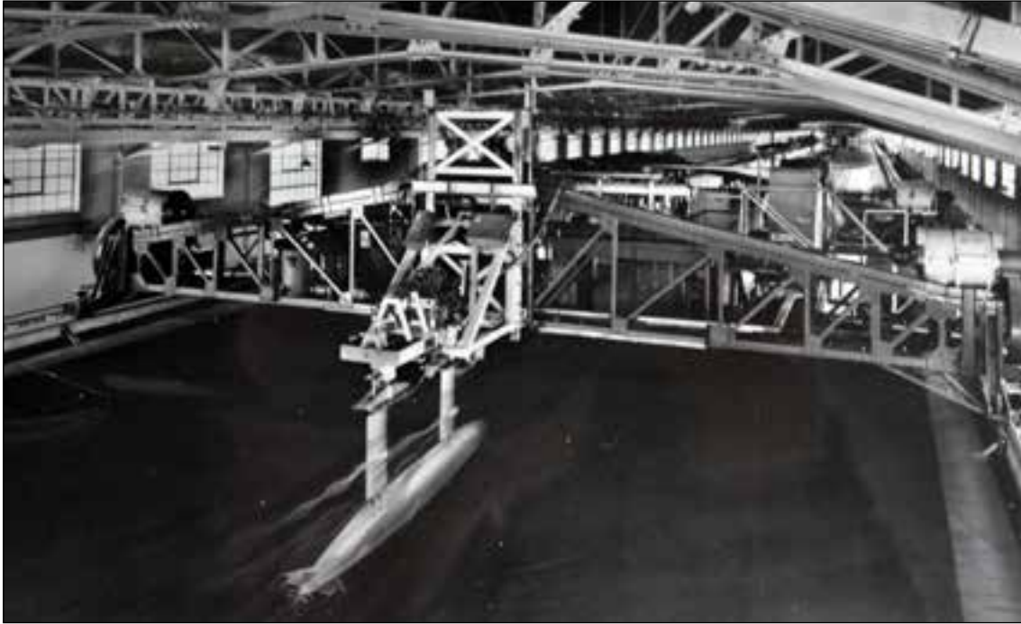
Figure 20: The carriage of No 2 Ship Tank following the addition of the Planar Motion Mechanism to allow a greater range of tests of model submarines (TNA ADM 226/1258)
