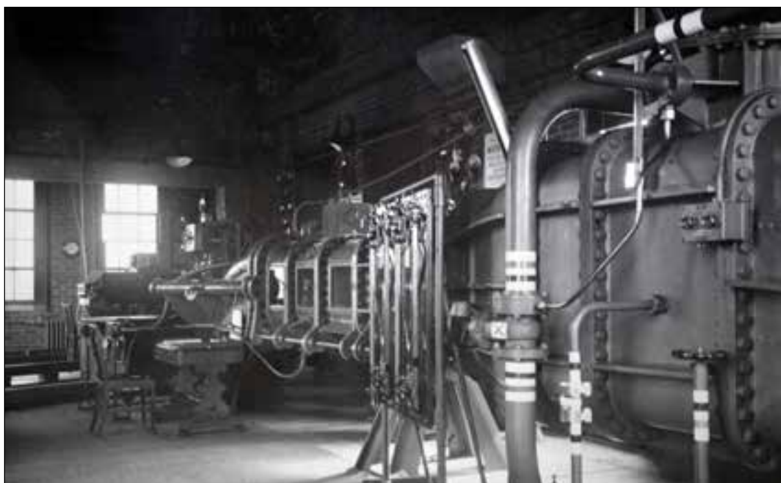
Figure 8: The upper limb and observation panels of No 1 Cavitation Tunnel (TNA ADM 1/23580)
