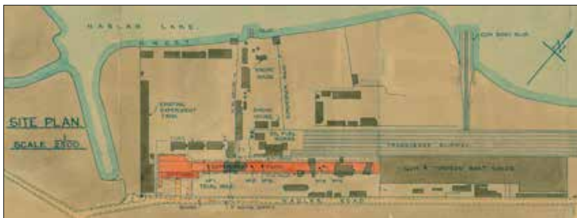
Figure 5: Plan of the AEW Haslar site in 1927 showing the location of the Liquid Fuel Experimental Station immediately to the north of the proposed No 2 Ship Tank highlighted in orange (HEA MD95/06498)
