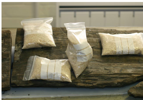
Figure 16: A timber during the re-attachment of some loose wooden fragments, which have been weighed down with rice-filled bags to achieve good adhesion
