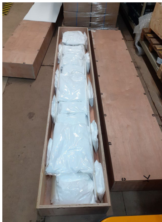
Figure 19: Timber 3 inside its Corex tray and with polystyrene foam beads in bags for extra support
