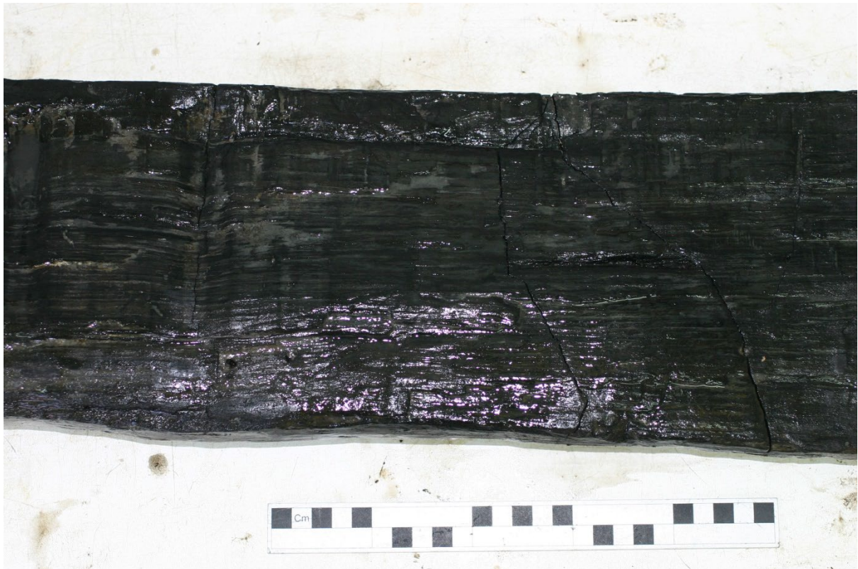
Figure 13: Large cracks running across the grain of Timber 3
