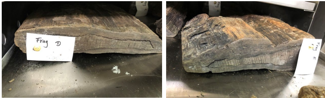
Figure 15: Splits along the interface of the well-preserved inner core and decayed outer layer, visible in the cross sections of Timber 3
