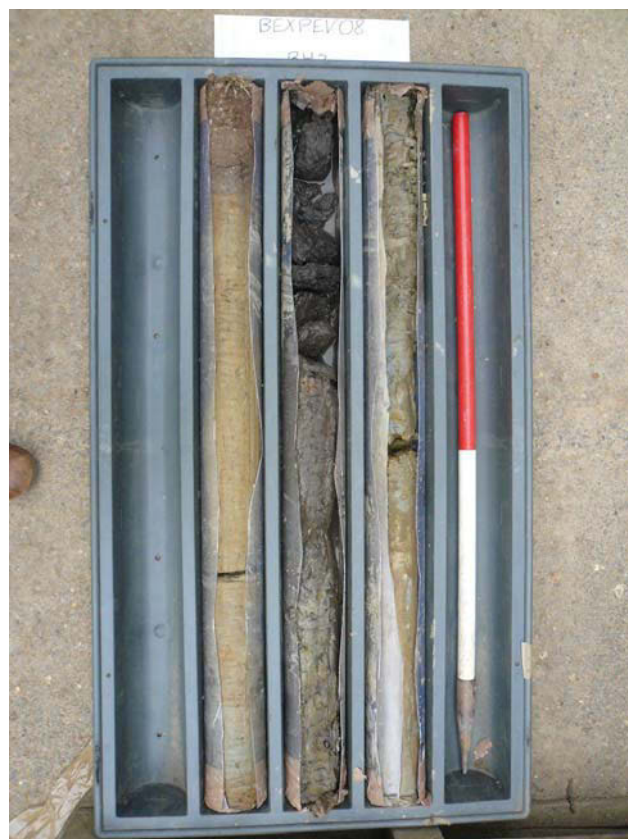
Plate 6: Borehole samples of the marsh sequence from the Pevensey Levels (1m scale)
