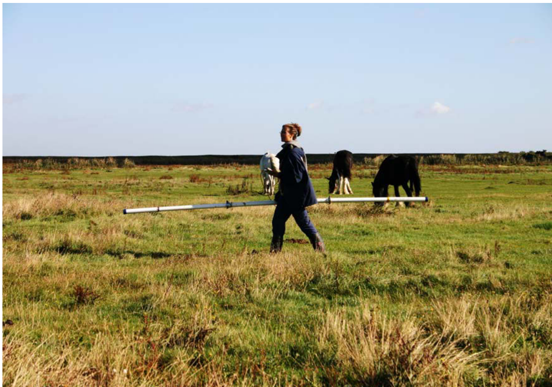
Plate 12: EM 31 survey being undertaken on reclaimed marshland
