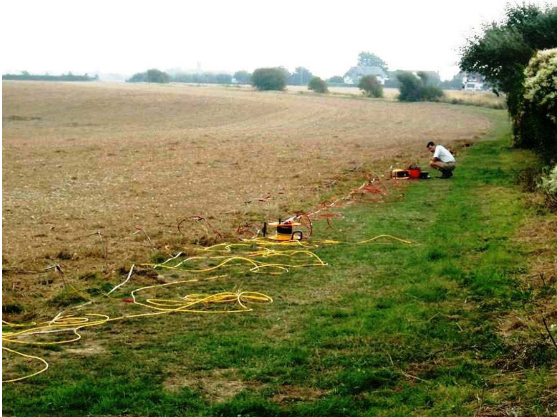
Plate 13: Undertaking resistivity profiling at London Gateway, Thames Estuary
