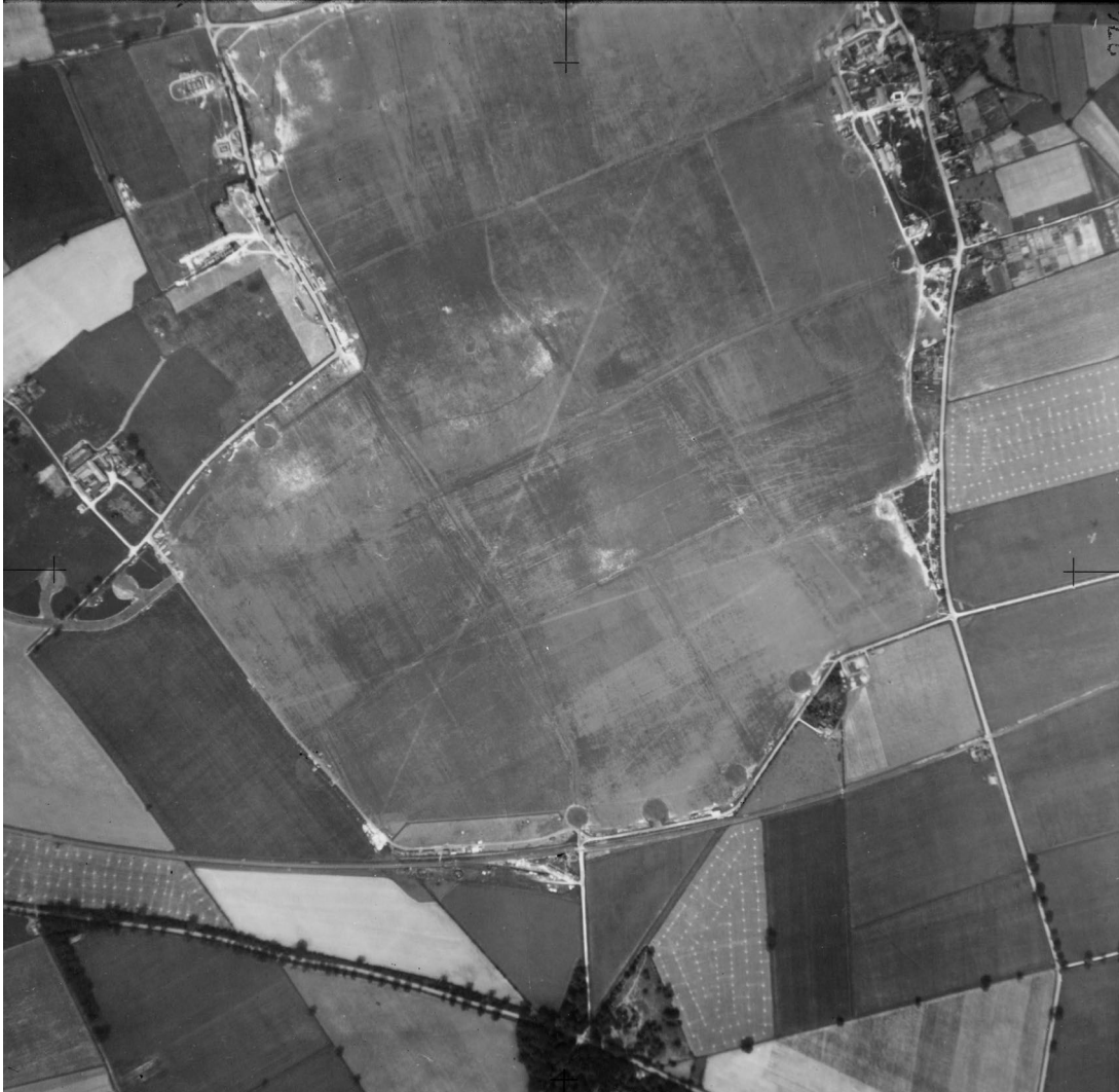
Figure 45 The early phase of RAF Oulton, photographed in 1942; at this stage the airfield had a grass landing ground, before the concrete runways were added after the site was redeveloped in 1943. Photograph: RAF/FNO/35 V 6063 02-JUL-1942 Historic England Archive (RAF Photography; detail).
