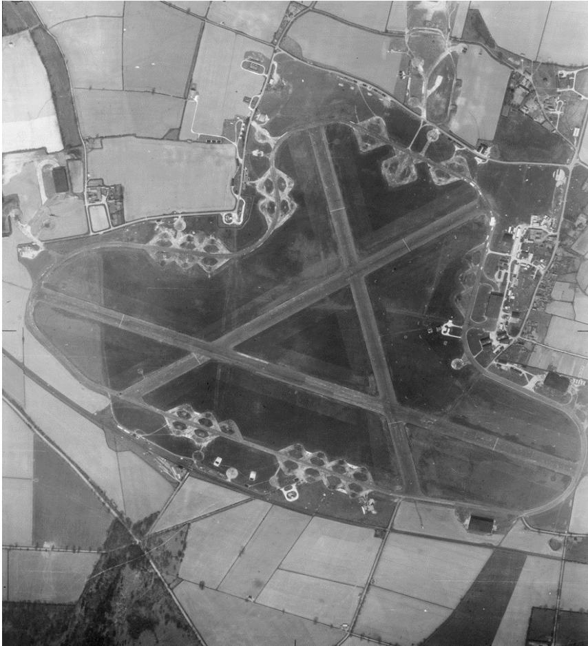
Figure 46 RAF Oulton in 1946, during its later phase; visible features include the T2 hangers, control tower, the technical site and the concrete runways. Photograph: RAF/106G/UK/1428 RS 4313 16-APR-1946 Historic England Archive (RAF Photography; detail).
