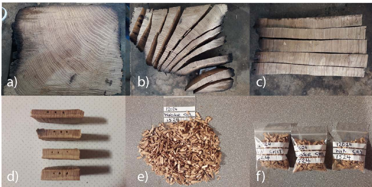
Figure 2. Dissecting single-ring tree-ring samples from timber 12024: a) original slice with ring-widths checked and selected rings marked out, b) slice split into wedges, c) wedges cut into slices, d) selected rings marked out on slices; e) chipped rings, f) bagged rings (photographs by R Howard).
