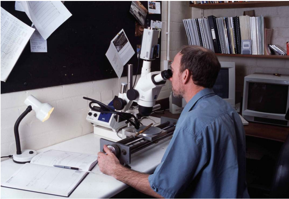
Figure A3: Measuring ring widths under a microscope. The microscope is fixed while the sample is on a moving platform. The total sequence of widths is measured twice to ensure that an error has not been made. This type of apparatus is needed to process a large number of samples on a regular basis
