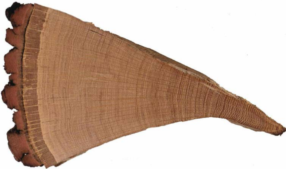
Figure A1: A wedge of oak from a tree felled in 1976. It shows the annual growth rings, one for each year from the innermost ring to the last ring on the outside just inside the bark. The year of each ring can be determined by counting back from the
