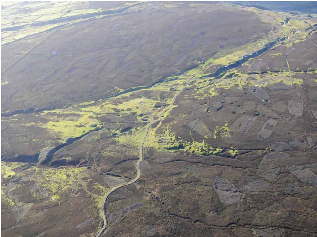
Figure 12.18 The Windegg vein runs diagonally across this image, the open cast working on the escarpment being just visible top right. The centre foreground shows an area of very small shafts known as Brass Pump Floats, probably exploiting a mineralisation deposit known as flats which followed near horizontal bedding of the limestone rather than a vein deposit. Recent alterations to the leat beside the shooting hut just above Brass Pump Floats revealed an extensive array of Mesolithic flints, a reminder that although this is perceived as a post-medieval mining landscape it contains evidence for a much longer history of land use. North Hush and Tanner Rake Hush are visible in the top left of the image, continuing to the right as the line of shafts along Cocker Vein (© English Heritage 16/12/2014 28645_047)
