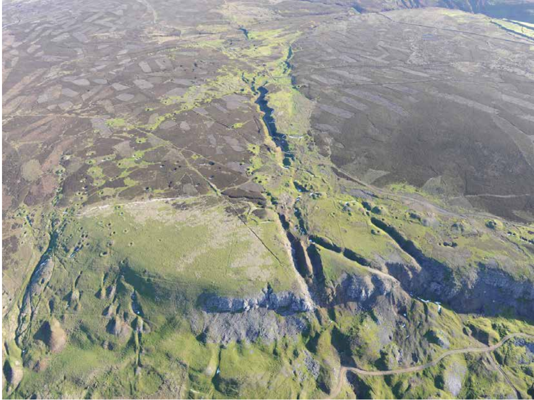
Figure 12.17 The Windegg escarpment is pierced by a series of open cast workings and unusually a series of small levels, clearly marked by the spoil heaps bottom left, which were probably, judging from their size, not very productive. The pockmarks on the plateau above the Tanner Rake Hush and Slei Gill is visible in the top right of the image, separated by a wide expanse of heather moorland (© English Heritage 16/12/2014 28645_042)
