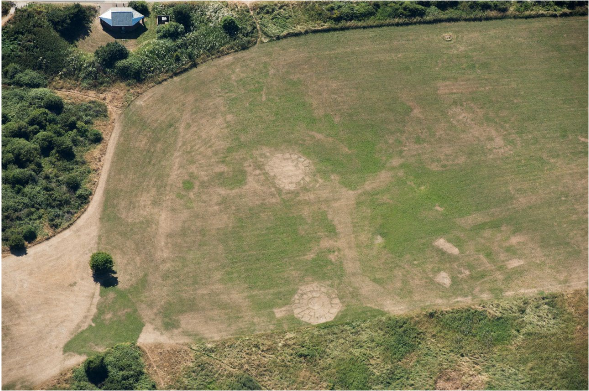
Figure 52: Cropmarks of the north-eastern and south-eastern gun emplacements at Gilkicker (Solent P3) HAA Battery on Stokes Bay (looking south). The buried reinforced concrete foundations of the octagonal gun holdfasts are visible, ringed by ammunition lockers and link by a paved road. HEA 33561_039 26-JUN-2018 Historic England ©Historic England Archive.
