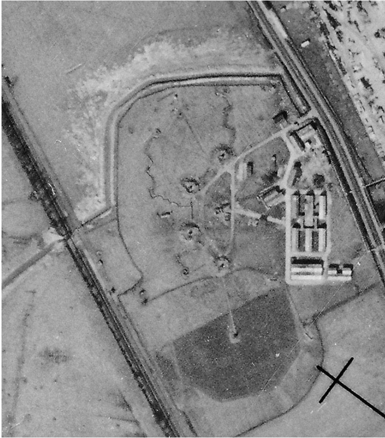
Figure 51a Aerial view of Holbrook (Solent P4) HAA gun emplacement with its octagonal false datum mat and central GL radar platform are visible to the south. (north to the top). Extract of RAF/HLA/426/RV 6041 24-MAR-1942 Historic England Archive (RAF Photography).
