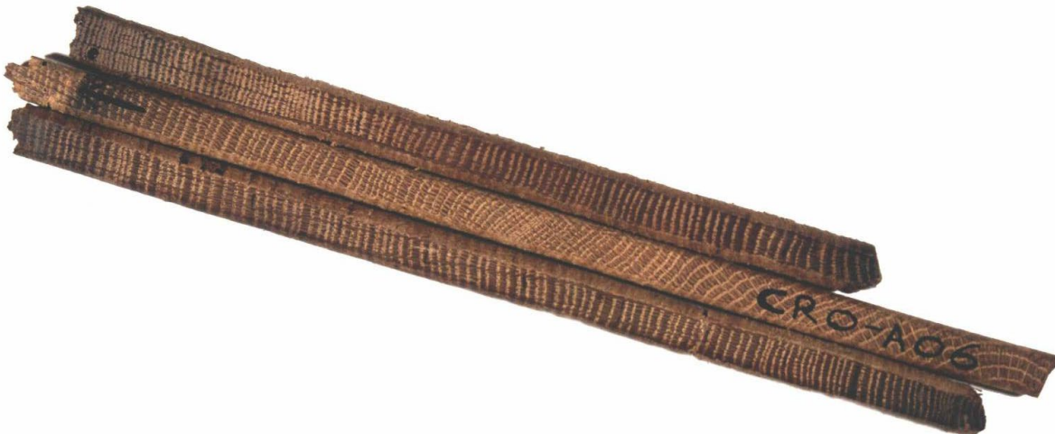
Figure A4: Three cores from timbers in a building. They come from trees growing at the same time. Notice that, although the sequences of widths look similar, they are not identical. This is typical.
