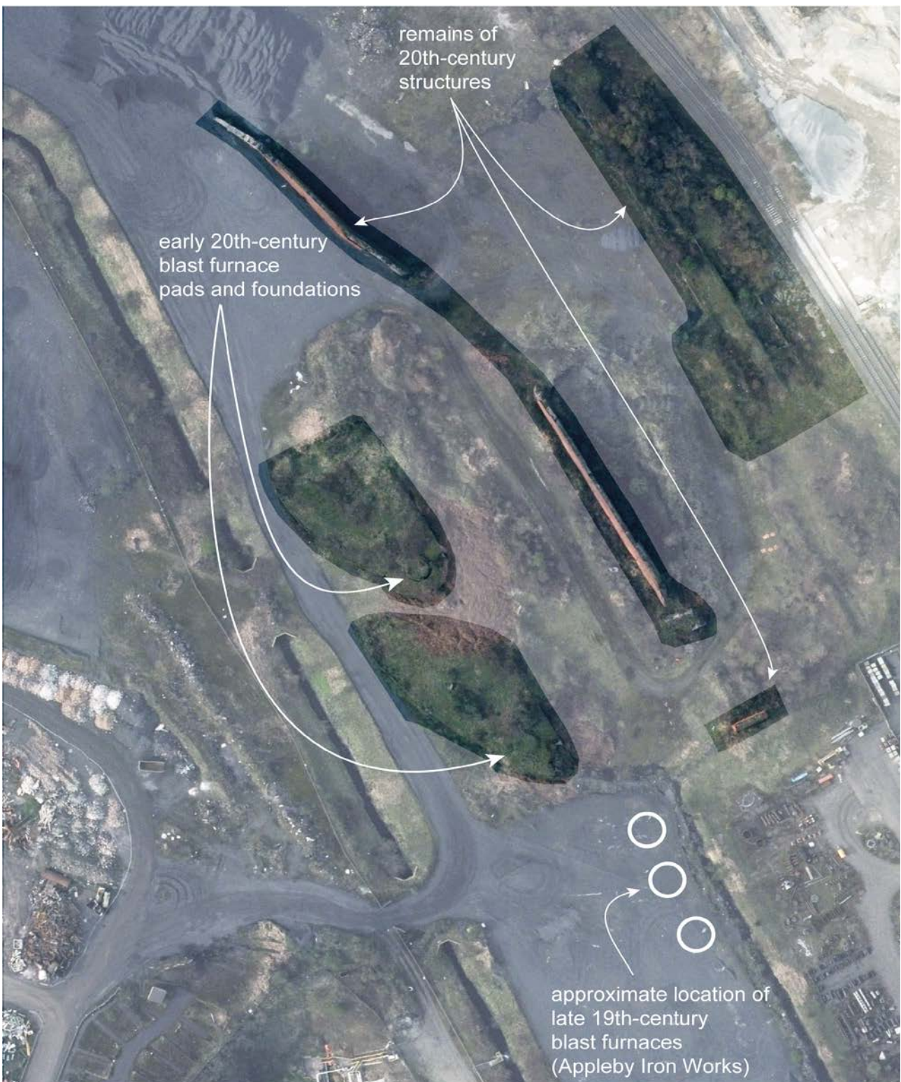
Figure 30: Earthworks and the low remains of structures on the site of the Appleby Iron Works (11 April 2022 © Bluesky International/ Getmapping PLC)
