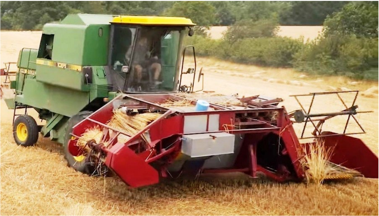
Figure 34: Combine-mounted reed comber and trusser harvesting stripped cereal straw.
