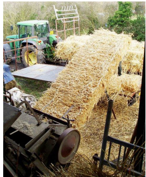
Figure 26: Low-density baler baling threshed LS and delivering bales onto a trailer.
