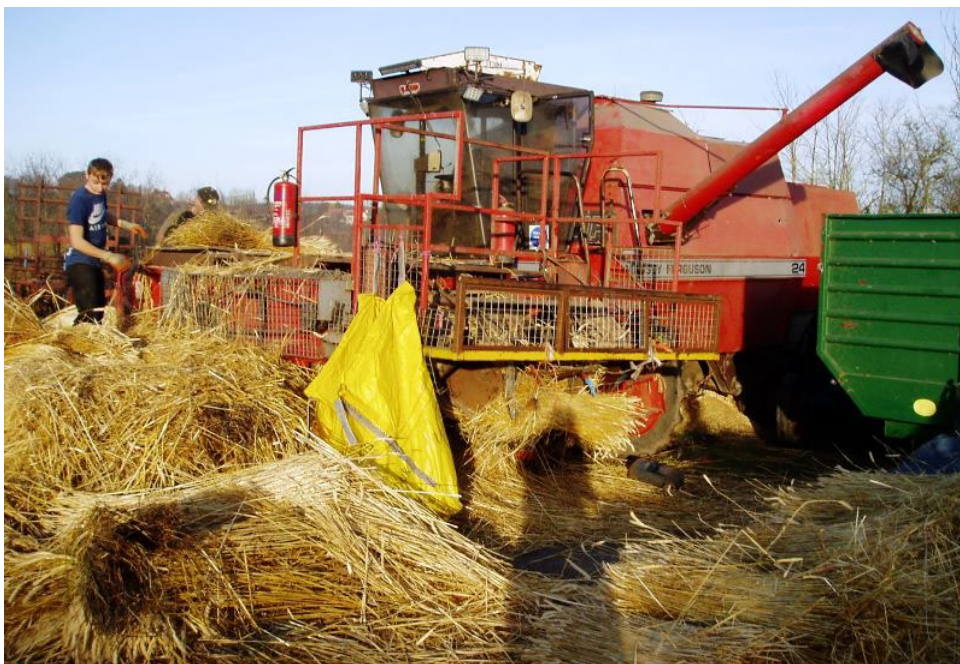
Figure 18: Bespoke reed comber (with integral trusser) fitted to a combine harvester.
