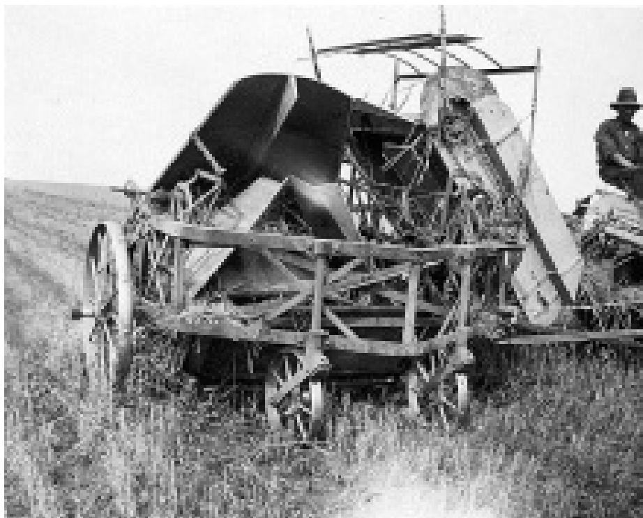
Figure 39: International Harvester Co. automatic stooker, c. 1926.
