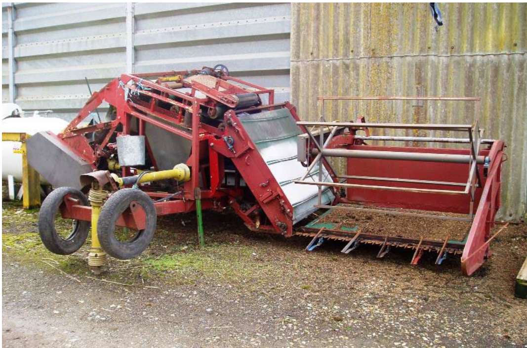
Figure 33: Bespoke tractor-drawn machine for cutting and binding stripped LS. It also removes residual grain from unthreshed or missed ears.
