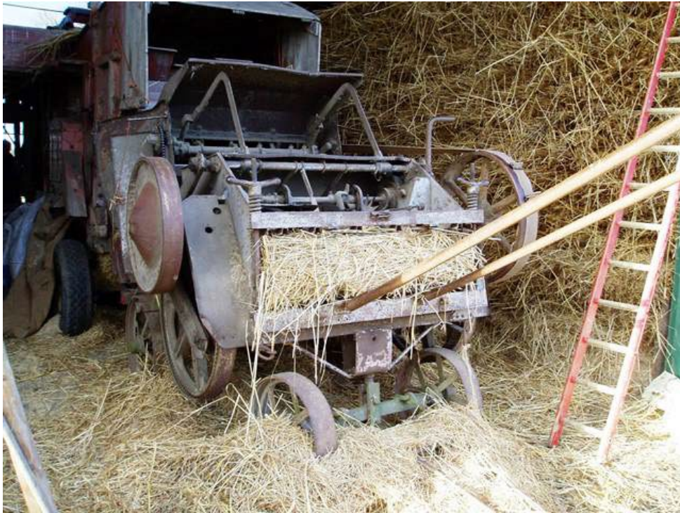
Figure 24: Low-density baler packaging LS from a threshing drum.
