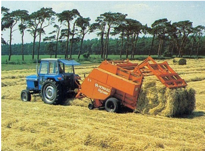
Figure 8: Howard Bigbaler baling straw after combining. NB: Not shown baling thatching straw.
