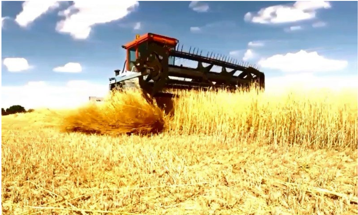
Figure 32: Adapted self-propelled swathing machine (swather) windrowing stripped wheat straw.
