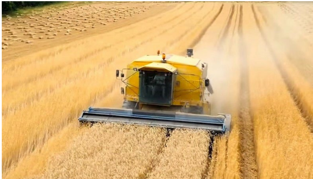
Figure 28: Grain removal from standing crop by combine fitted with a stripper header.
