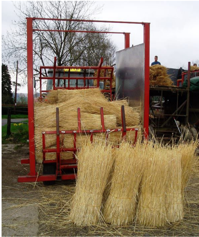
Figure 21: Hydraulically operated packaging cage being loaded with CWR trusses.
