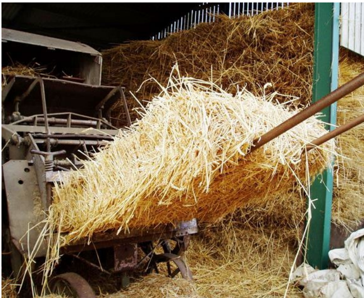
Figure 26: Low-density baler baling threshed LS and delivering bales onto a trailer.
