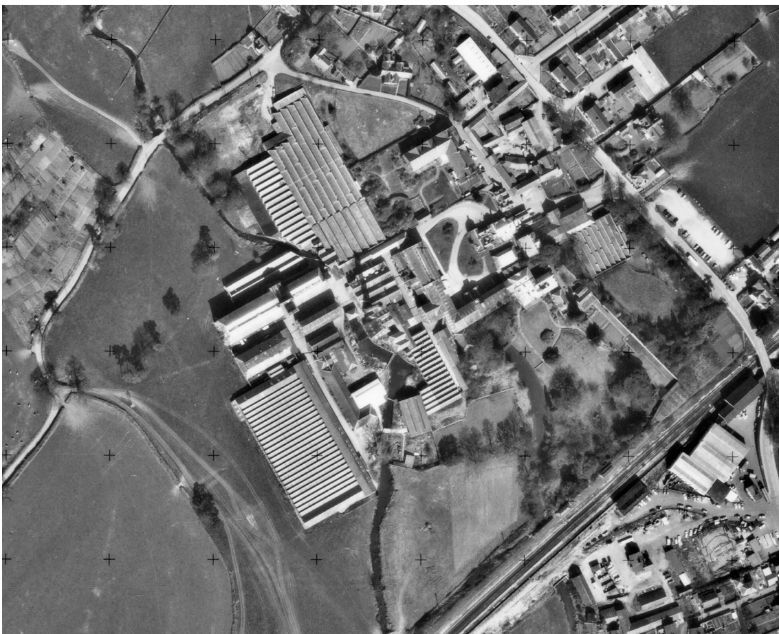
Figure 27: Tonedale Mill in 1973, with north at the top. The course of the Back Stream (left/west) and Mill Head (right/east) can be seen flowing from the south up into the mill complex. Note the purposefully widened stretch of the Mill Head as it passes through the large garden on the south side of Tonedale House. [OS/73039_006 29-MAR-1973 © Crown copyright. Historic England (OS Photography)]
