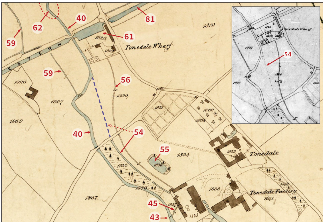
Figure 36: Extract from the Wellington tithe map of 1839. The postulated continued course of the tailrace [54] has been added as a dashed blue line and can be seen depicted on an alternative copy of the tithe map, shown as an inset. Parallel to its east is the narrow channel [56] from Tonedale Mill to the wharf and former pond [55], and to the west the Back Stream [40]. Not reproduced at scale. [main map SHC D/D/rt/M/367, accessed via the 'Know Your Place' website, reproduced with kind permission of the South West Heritage Trust; inset map © Crown copyright images reproduced courtesy of The National Archives]
