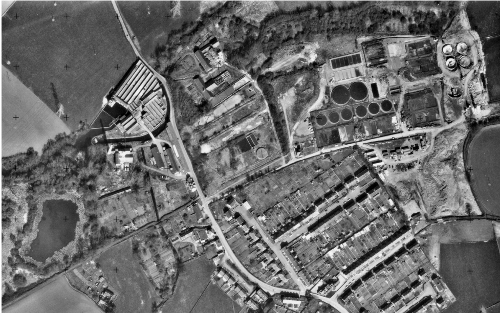
Figure 57: Tone Works in 1973, with north at the top. Additional long settling tanks now occupy the formerly open area to the south of the grease works (centre) and, east (right) of this, the later sewage works with its settling tanks have expanded. [OS/73039 006 29-MAR-1973 Historic England (OS Photography)]
