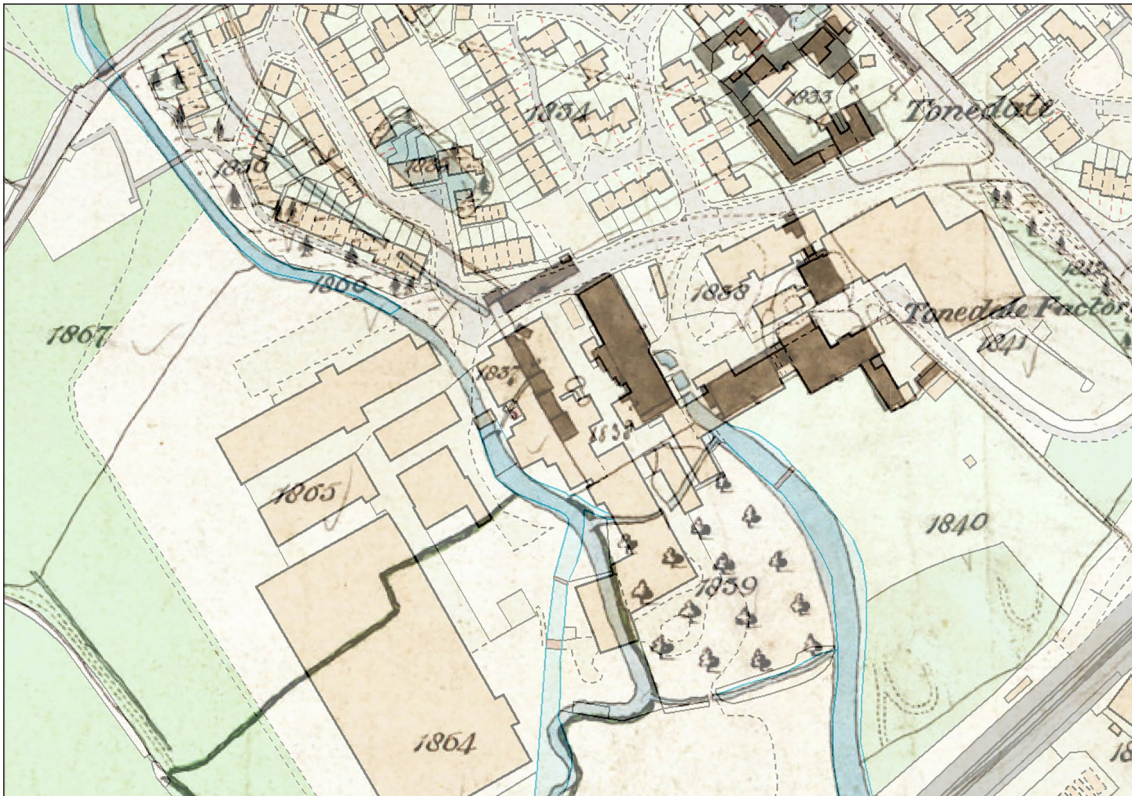
Figure 29: Earlier routes of water features through Tonedale Mill, illustrated by overlaying the 1839 Wellington tithe map on the modern OS Mastermap data. Cross-channel [51] can be seen connecting the two main watercourses immediately south of the early factory buildings. The former distinct bend in the Back Stream [52] (bottom centre) had been straightened by 1888, and most of the other features were culverted as the site developed and expanded. Not reproduced at scale. [Background mapping © Crown Copyright and database right 2023. All rights reserved. Ordnance Survey Licence number 100024900 © Historic England | overlay source: SHC D/D/rt/M/367, accessed via the 'Know Your Place' website, reproduced with kind permission of the South West Heritage Trust]
