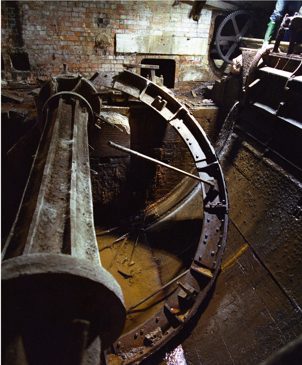
Figure 46: The waterwheel and pit [72] at Tone Works, photographed in October 1995 [Peter Williams © Crown copyright. Historic England, AA96/00684]
