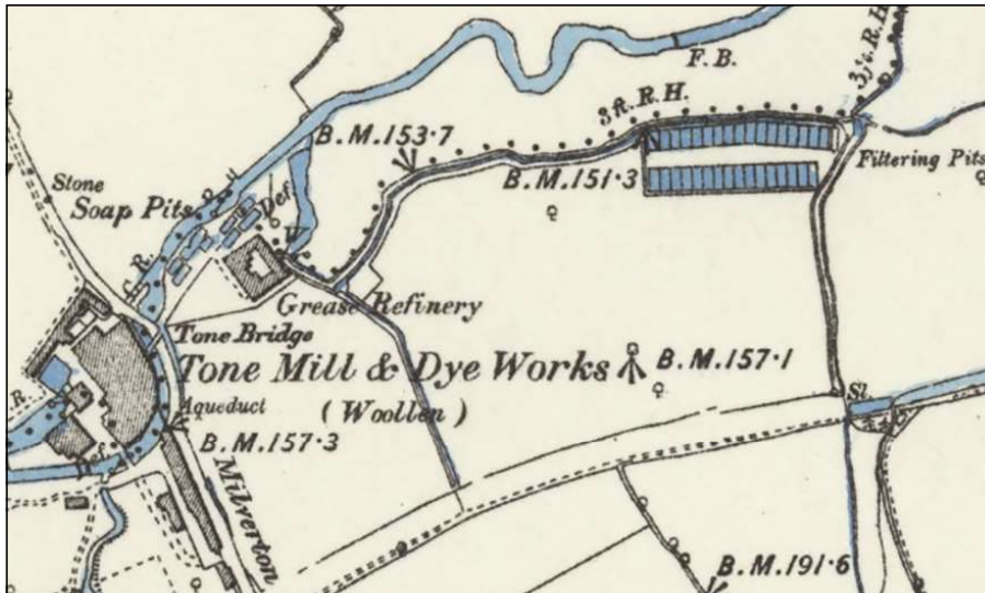
Figure 53: Extract from the coloured 1888 OS 25-inch map showing Tone Works ('Tone Mill & Dye Works') and adjacent grease works ('Grease Refinery') with its rectangular 'Soap Pits' for lanolin extraction and a channel taking wastewater to two rows of 'Filtering Pits' to the far east of the site. Not reproduced at scale. [Reproduced with the permission of the National Library of Scotland]
