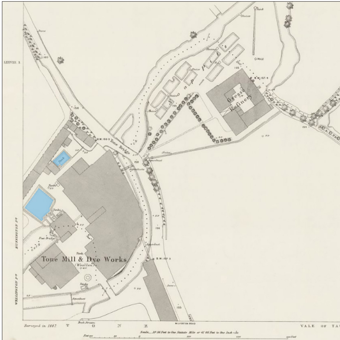
Figure 50: Water tank [67] and smaller tank [69] at Tone Works, highlighted in blue, and the grease works with its soap pits, shown on the OS 1:500 Town Plan of 1888. Note that the dotted line of the parish boundary follows the earlier course of the river where it used to bend tightly before it was modified to reduce flooding and increase land for building. Not reproduced at scale. [Reproduced with the permission of the National Library of Scotland]
