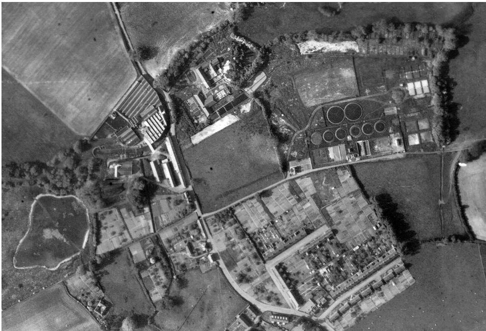
Figure 56: Vertical view of Tone Works in 1946, with north at the top. The finishing and dyeworks on the west (left) of the road and the grease works with its rectangular settling tanks to the east (right). The later sewage works is located to the south and south-east. [RAF/3GTUD/UK/207/ PT1 5001 13-MAY-1946 Historic England Archive (RAF Photography)]
