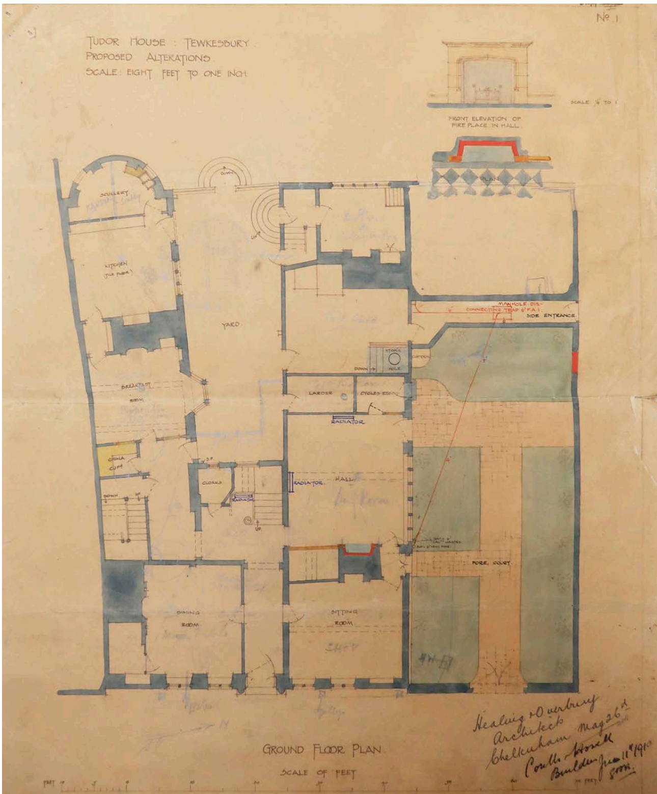
Figure 10: Contract drawing of the ground floor as proposed, by Healing & Overbury, May 1910. The room names in pencil were those used by the hotel in 1934. North is to the right. [Gloucestershire Archives, D5587/box9627, item 13/27]
