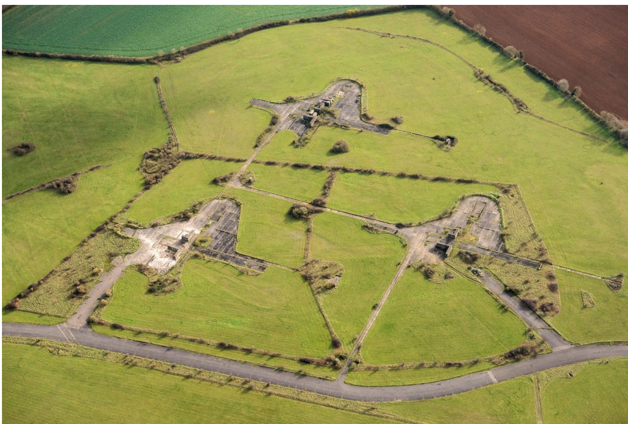
Figure 24: The remains of the Cold War Thor missile complex at North Luffenham. The outlines of the underlying Second World War airfield frying pan and spectacle loop dispersals are visible in the grass. 33983_014 12-Nov-2020 © Historic England Archive.
