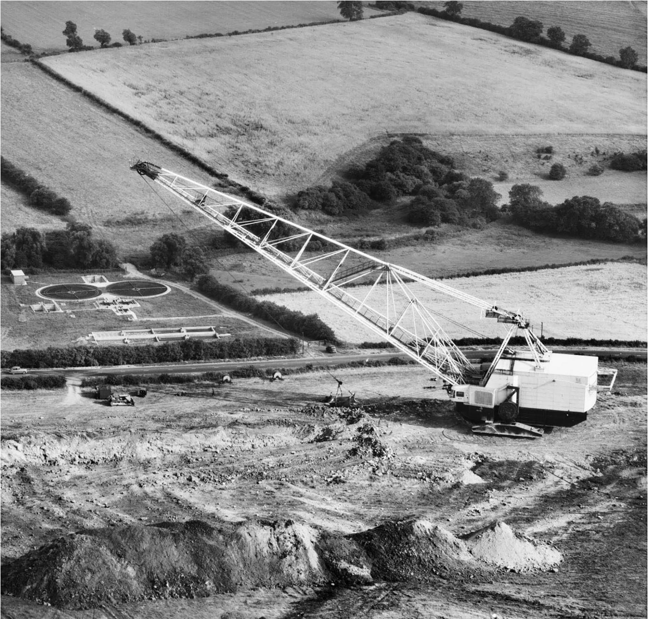
Figure 31: A working walking dragline quarrying ironstone off Stamford Road, Weldon near Corby in 1953. EAW051406 1953. © Historic England Archive
