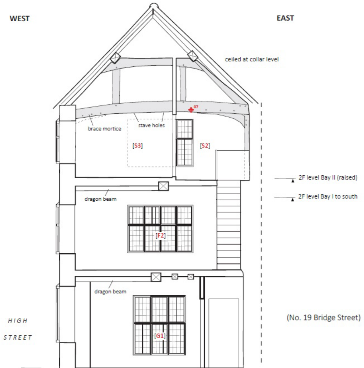
Figure 3: Section through truss one (T1) showing the location of sample 07 [adapted from an original drawing by Ric Tyler]
