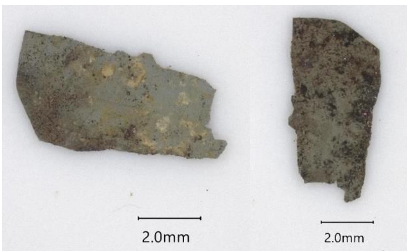
Figure 26: Optical images of the paint sample from the cockpit floor structure of Fairey Barracuda LS931 showing grey/green paint.
