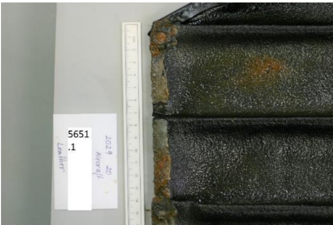
Figure 8: Part of the seat component 5651.1, leather (flesh side) with latex around the periphery.
