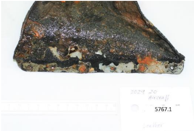
Figure 13: Paint adhering to the leather on 5767.1.
