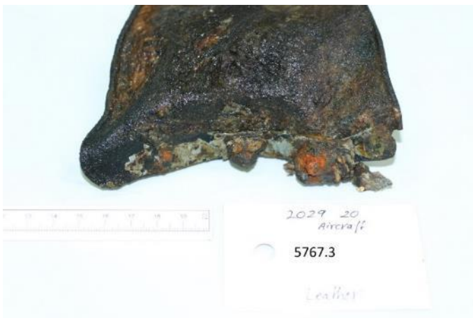
Figure 15: Paint adhering to the leather on 5767.3.
