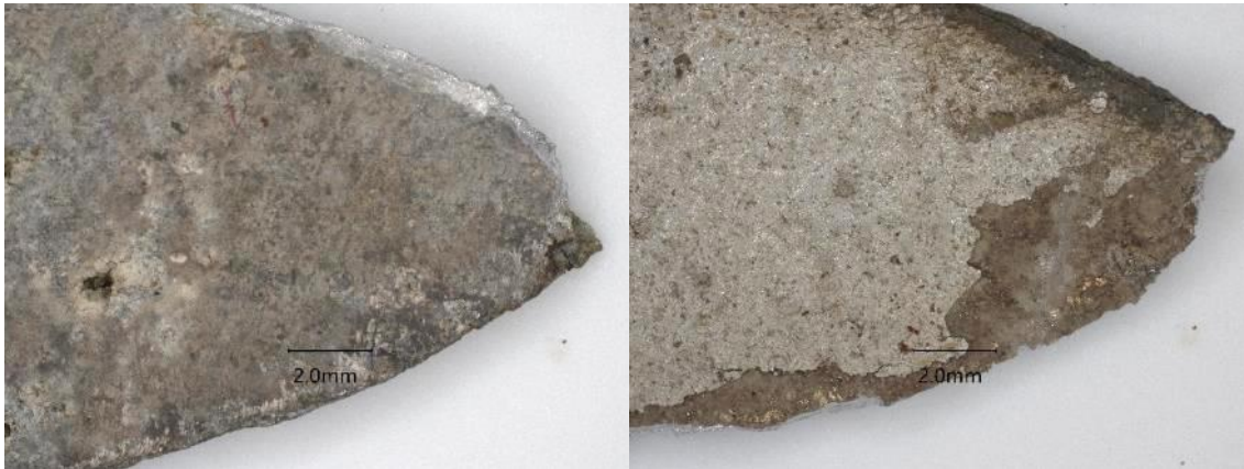
Figure 27: Optical images of a piece of painted metal from the cockpit floor structure of Fairey Barracuda LS931, with grey paint on both sides and an additional silver layer on one side (right).
