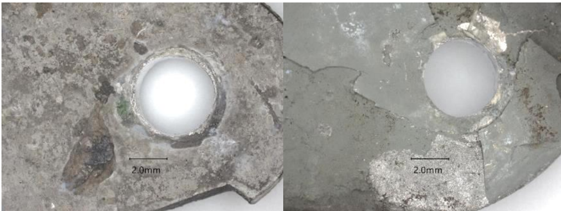
Figure 25: Optical images of the metal from the cockpit of Fairey built Barracuda PM870 showing the grey/green paint, metallic substrate and small area of green pigmented topcoat paint on one surface (left).
