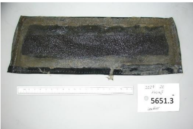
Figure 9: Part of the seat component 5651.3, leather (flesh side) with latex around the periphery.
