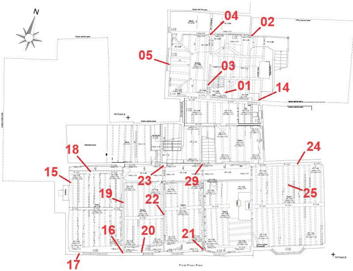
Figure 4: Plan of the first floor showing the positions of the timbers sampled for dendrochronology [© owner; adapted from an original drawing by BES Geomatics]
