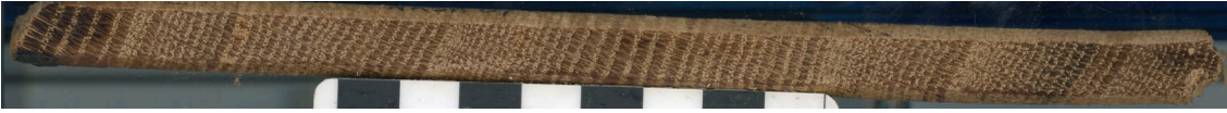
Figure 5: Scan of sample nash07 showing multiple bands of narrow rings, in which some of the ring boundaries could not be reliably distinguished.
