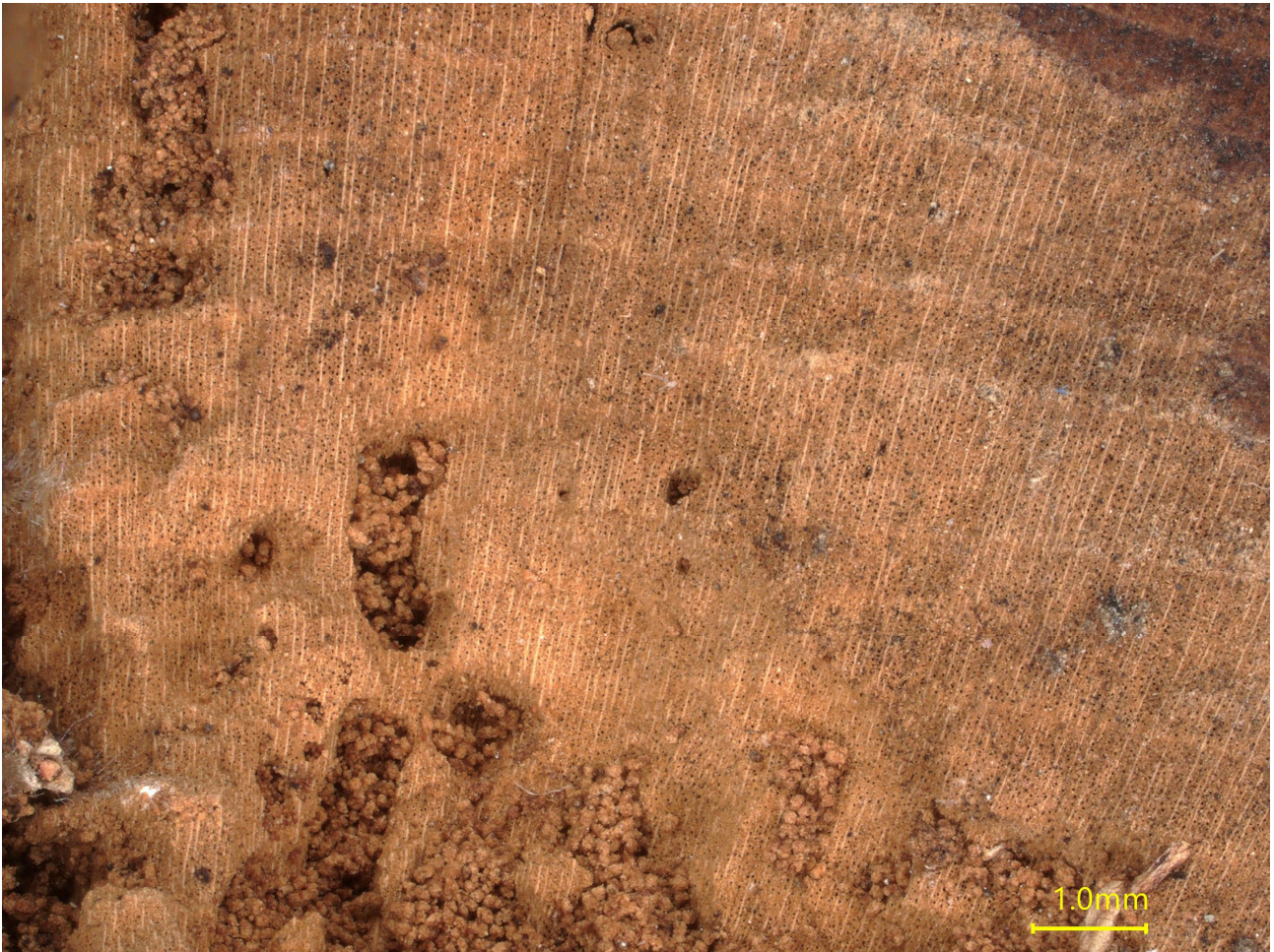
Figure 3: Image of an exposed, eroded face of the wooden ball, showing frass-filled insect tunnels. Image: Z. Hazell © Historic England.
