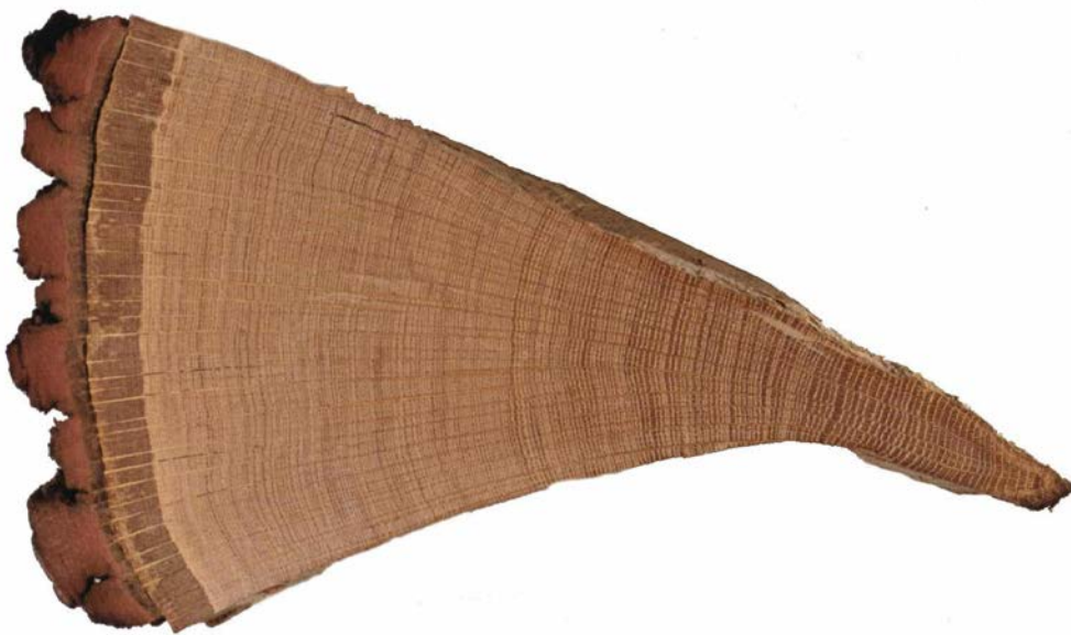
Figure A1: A wedge of oak from a tree felled in 1976. It shows the annual growth rings, one for each year from the innermost ring to the last ring on the outside just inside the bark. The year of each ring can be determined by counting back.
