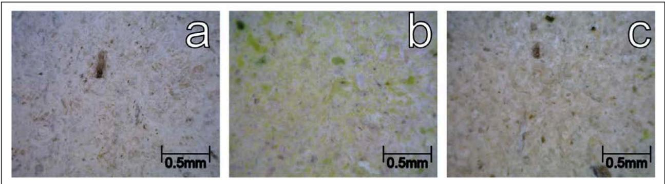
Figure 8: Unweathered Jordans Basebed limestone samples taken at 50x magnification: (a) without algal growth, (b) with algal growth, (c) post sampling.
