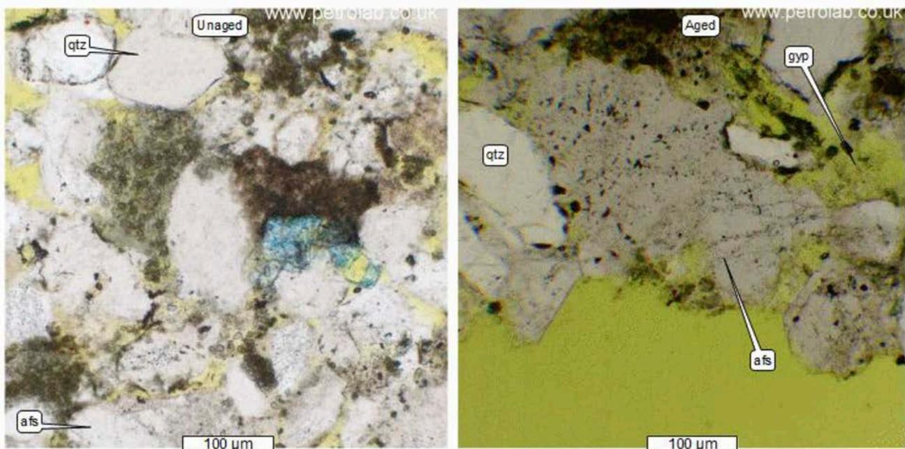
Figure 3: Howley Park sandstone sample from the petrography report. The sample referred to as 'unaged' is the unweathered sample; the 'aged' sample is artificially weathered. Key: qtz = quartz, afs = alkali feldspar, gyp = gypsum.
