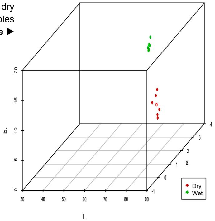
L\*a\*b\* colourimetry of wet and dry untreated stone samples
