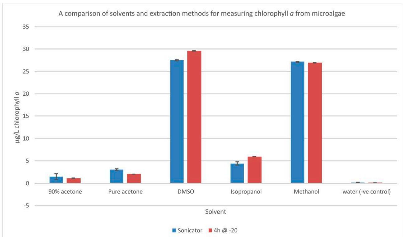
Figure 7: A comparison of solvents and techniques for extracting chlorophyll *a* from terrestrial algae. Using DMSO followed by freezing generated the highest amount.
