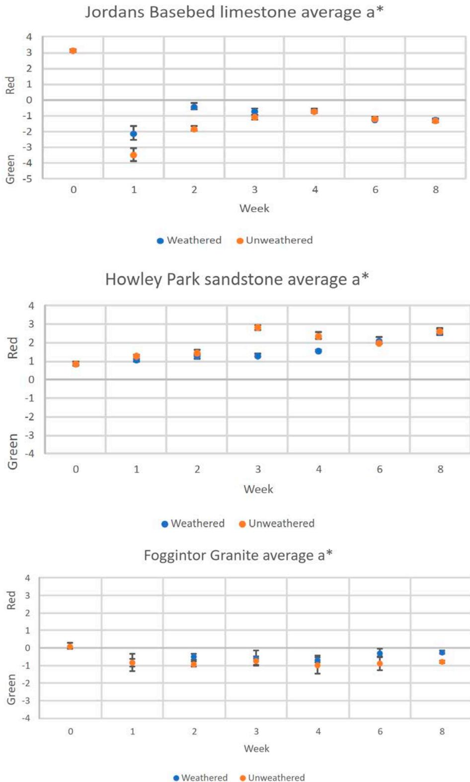
Figure 10: Average a\* plotted over 8 weeks for unweathered and weathered samples of Jordans Basebed limestone, Howley Park sandstone and Foggintor granite.
