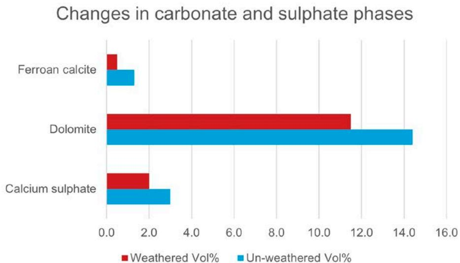
Figure 5: Changes in the carbonate and sulphate phases after artificial weathering in Howley Park sandstone.
