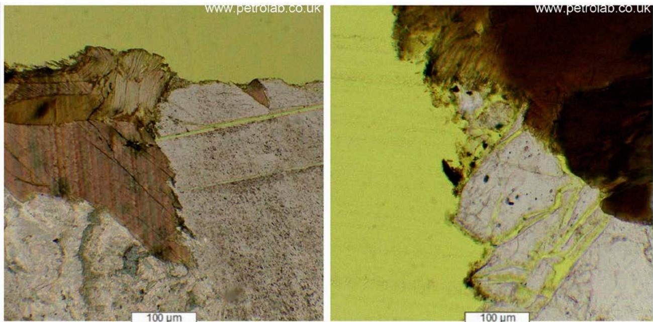
Figure 6: Plane polarised light microscopy of Foggintor granite from the petrography report. Unweathered (left) and artificially weathered (right) samples demonstrate the increase in fracturing, in this case in the biotite mica crystals.
