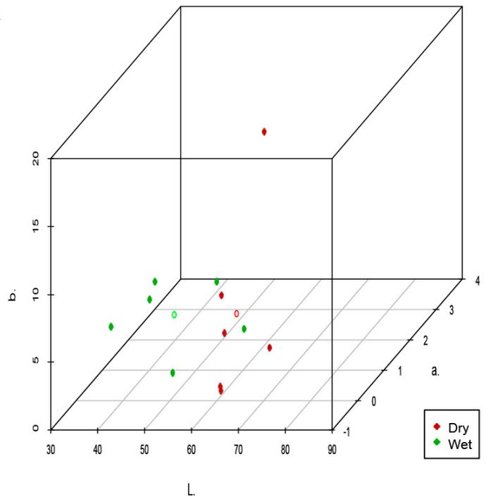
L\*a\*b\* colourimetry of wet and dry untreated stone samples
