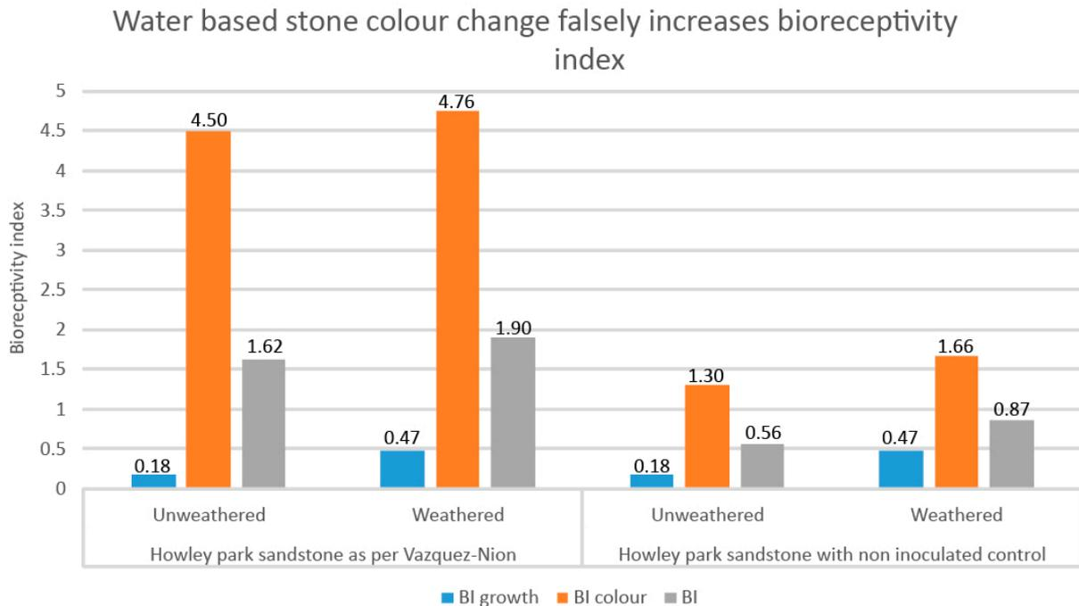
Figure 12: Comparison of bioreceptivity index calculations based on Vázquez-Nion *et al*'s original paper and our modified version. This clearly shows that water-based stone colour change causes an artificial increase in the bioreceptivity measurements for Howley Park sandstone.
