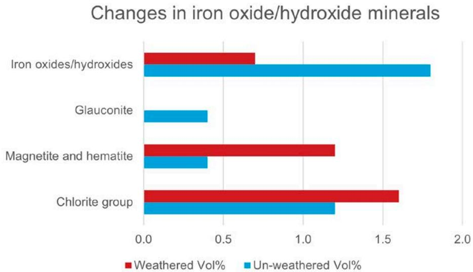
Figure 4: Changes in the iron oxide/hydroxide minerals after artificial weathering in Howley Park sandstone.
