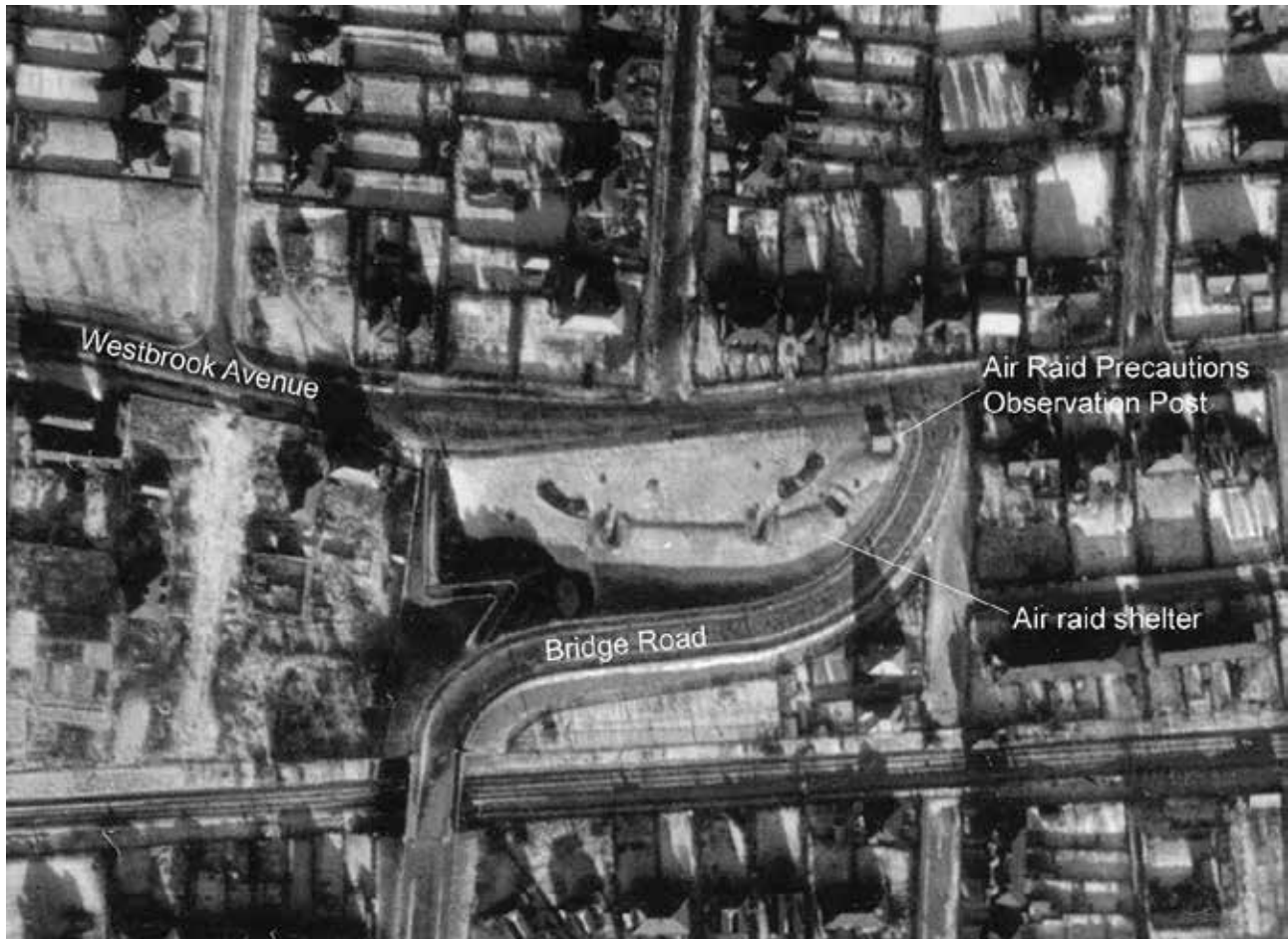
Figure 127: Large curved public air raid shelter with three separate entrances on open ground at Westbrook Avenue, Westbrook. [Extract of RAF/26J/BR194 VC 12 10-JAN-1941. Historic England Archive (RAF Photography)]
