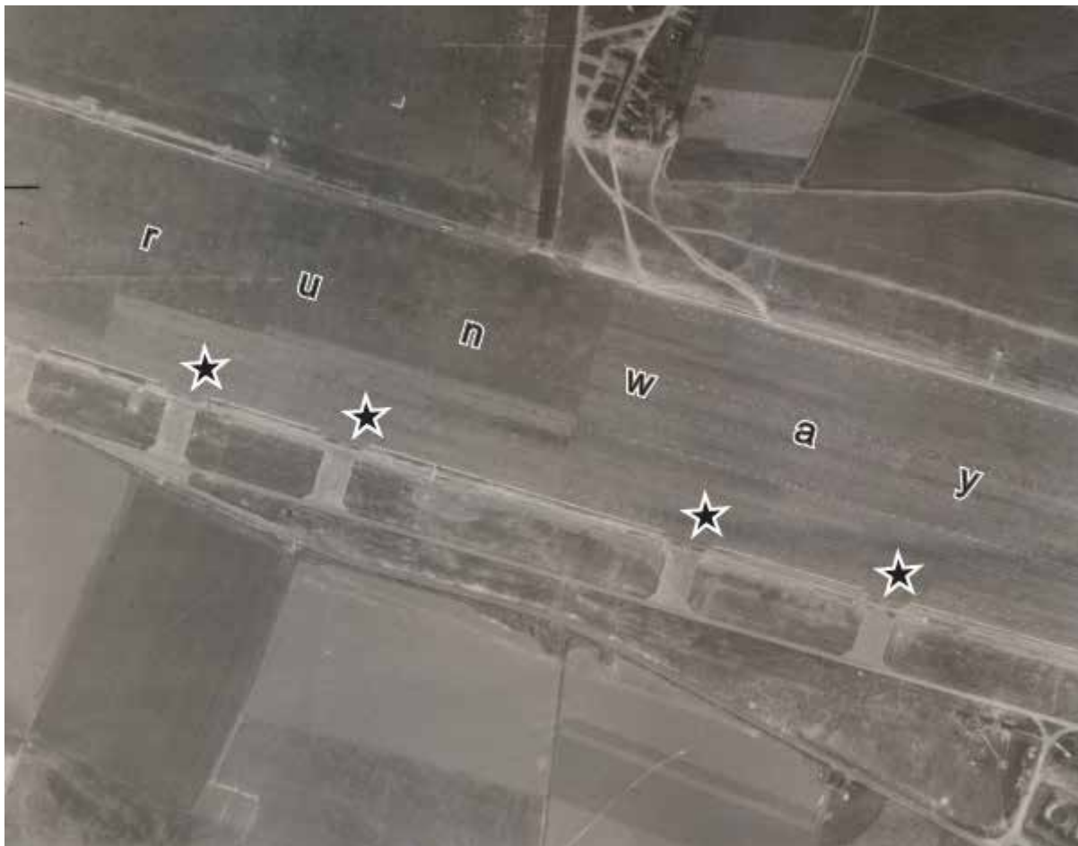
Figure 98: Scorching on RAF Manston salvage bay entrances resulting from FIDO burns (indicated by stars). North at top, unscaled extract from RAF/106G/UK/1378 V 5076 04-APR-1946. [Historic England Archive (RAF Photography)]
