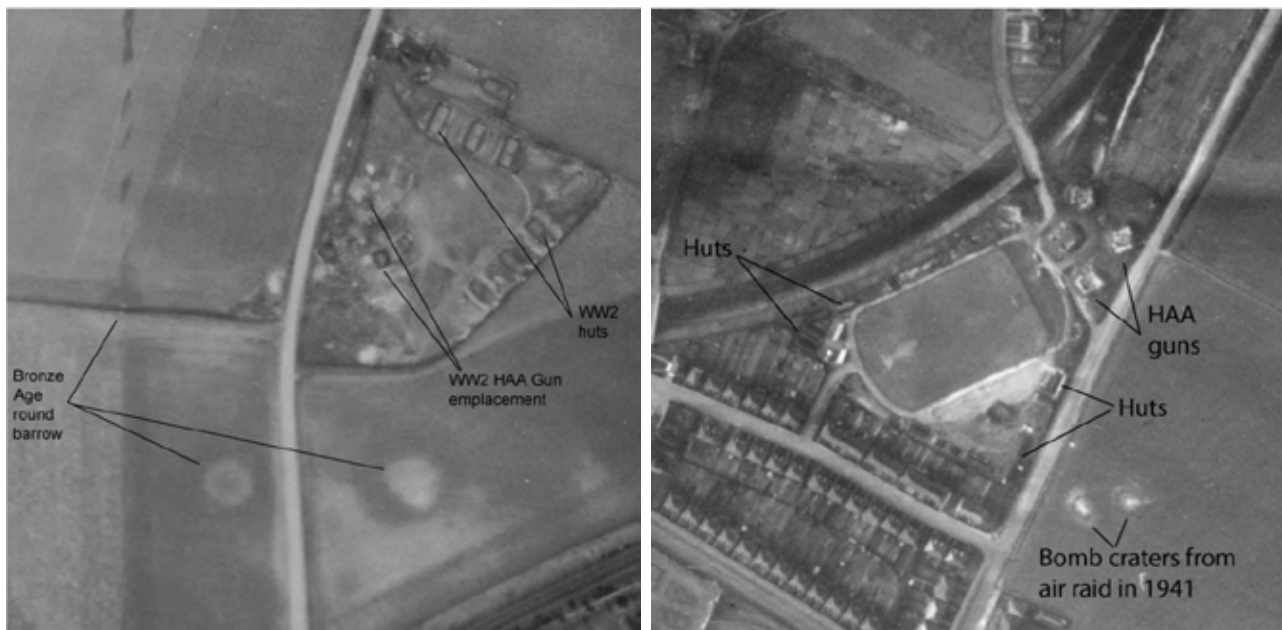
Figure 124: HAA batteries at Ozengell Grange and at Dumpton sports ground. [Extracts from RAF 106G/UK/1378 V 5069 04-APR-1946 and RAF/HLA/386 RS 912 02JAN-1942. Historic England Archive (RAF Photography)]
