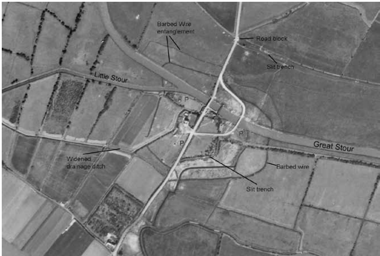
Figure 116: Defended locality at Plucks Gutter river crossing. (P marks the location of pill boxes. [Extract of US/7PH/GP/LOC295 V 5005 20-APR-1944 Historic England Archive (USAAF Photography)])
