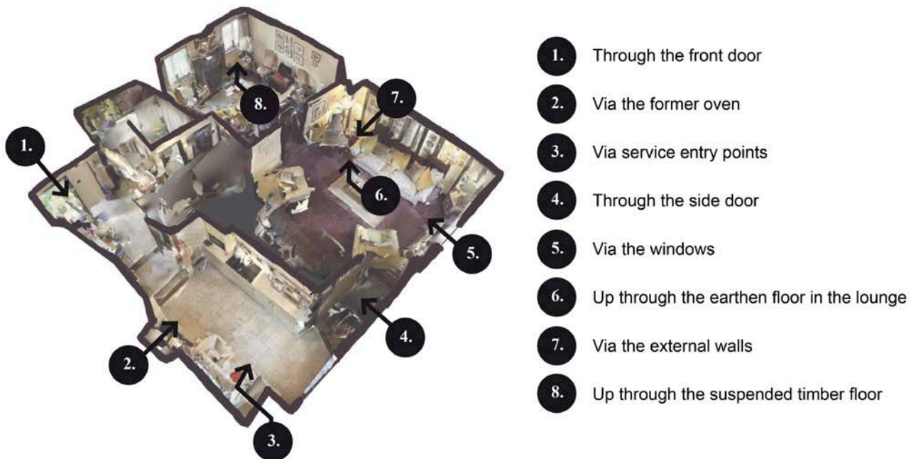
Figure 11: Floodwater entry points © The Environmental Design Studio
